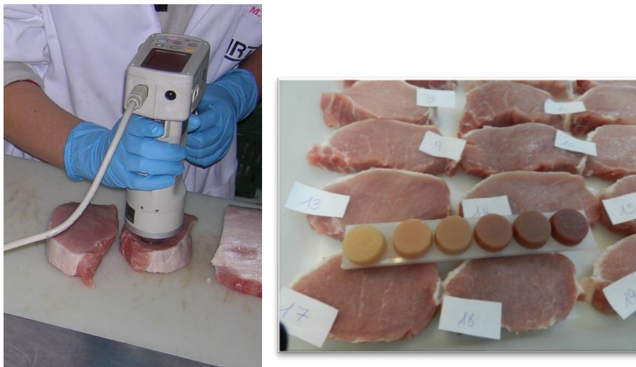
Figure 10. Colour measurement with the colorimeter Minolta (left) and the Japanese Scale of Colour (right).
