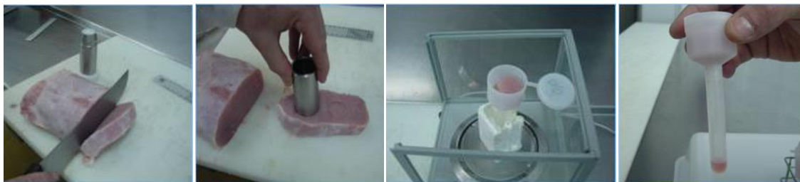
Figure 11. Drip loss determination.
