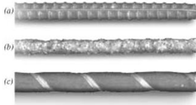
Figura 9. Tipus d'acabats superficials: (a) ribbed ; (b) sand-coated ; (c) wrapped (ACI 440.1R-06)
