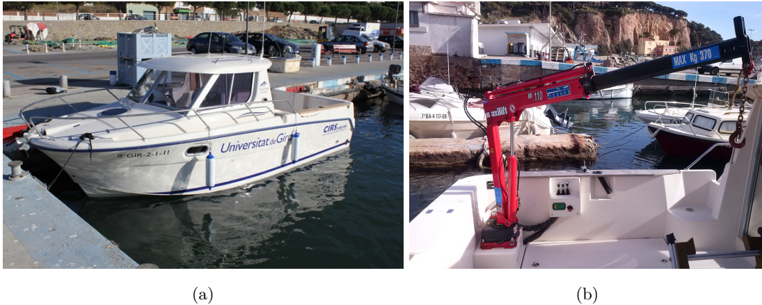
Figure 1.2: The Sextant research vessel. (a) Shows an overall view of the 7 meters long vessel. (b) A crane is used to deploy and recover the robots.
