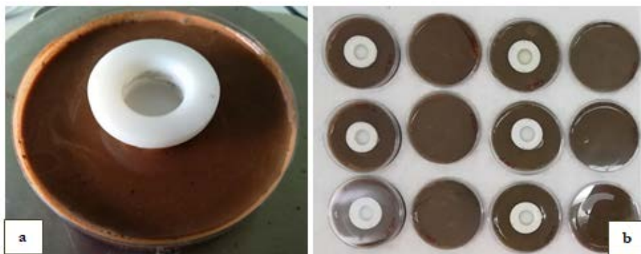
Figure 6.1: a) DGT sampler deployed in the soil sample. b) DGT devices per triplicate for every soil sample.
