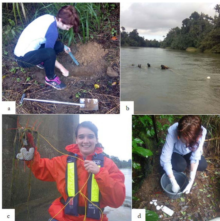
Figure 5.2: a) Soil samples collected b) DGT deployment in Tully river c) DGT devices in the plastic basket d) Water samples collected.
