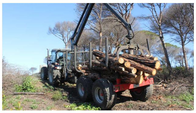
FIGURA 6. Clearing on road by tractor and light self-loading trailer. Image: P. Pons.
