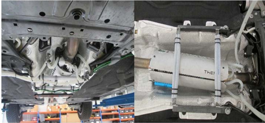
Fig. 6. Details of the ATEG installed on the exhaust system of the engine cell.
