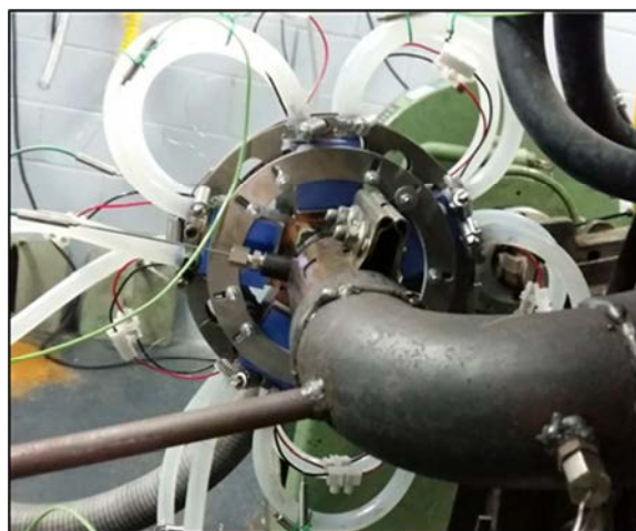
Figure 1.4: Radial ATEG XUD7/K engine installed.
