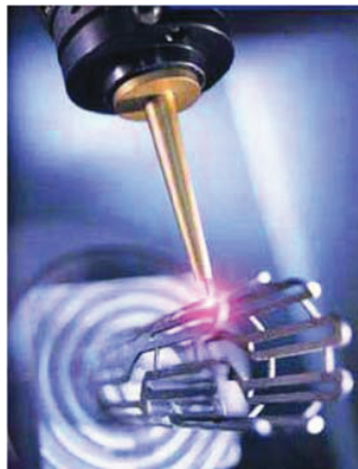
Figure 2.15. Laser Cutting Process of Stents
