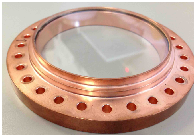
Figure 9: Scheme for the operation of PMTs in a helium-rich atmosphere ( top figure). The PMT itself remains at vacuum looking into the active volume through a crystalline quartz/sapphire window that can be coated with a wavelength shifter to maximize the light transmission. The crystal is welded to a metallic frame that can easily be mounted in a flange with a metallic sealing, avoiding helium diffusion into the PMT volume. The bottom figure shows one of the NEXT-NEW PMT protective windows. A similar concept can be applied for operation within a helium atmosphere using a metallic sealing for this frame.
