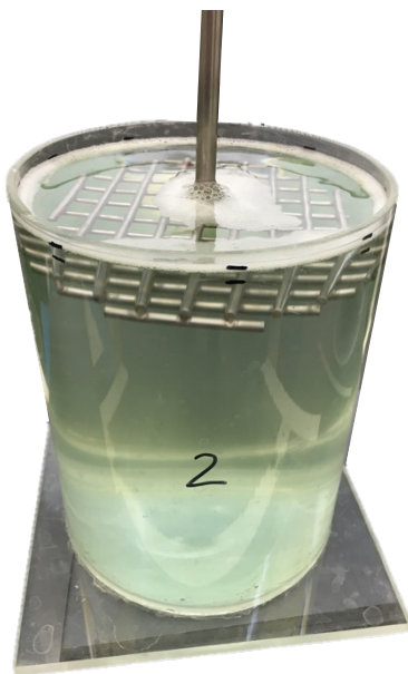
Fig. 2. Image of one of the three Plexiglas containers used for the experiments along with the oscillating grid.
