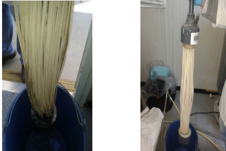
Figure 3. 2. Membrane before cleaning (left) and after cleaning (right)
