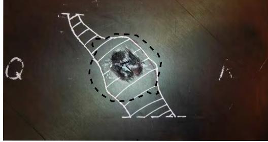
Fig. 6.10: Zoomed view from the impacted side after the LVI. The white dashed area is the experimental projected delamination area ( A_d = 1575 \text{ mm}^2 ) while the dark dashed line is the contour of the numerical projected delamination area ( A_d = 1246 \text{ mm}^2 ).
