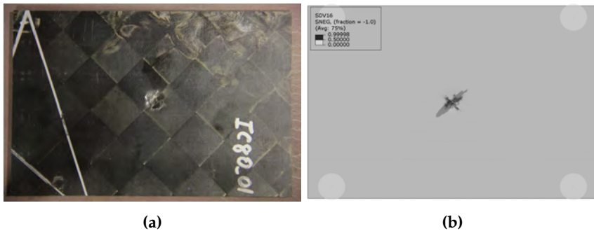
Fig. 5.18: Front - face view (30 J) at (a) specimen and (b) numerical model. Field output of fiber damage variable (SDV16) with applied translucency.
