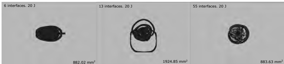
Fig. 5.28: Effect of the number of interfaces considered for delamination on the projected delamination area for the 20 J impact. Contour plot of the cohesive elements with d = 0.9 up to fully damage.
