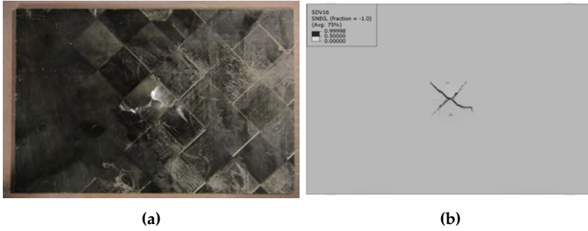
Fig. 5.19: Back - face view (30 J) at (a) specimen and (b) numerical model. Field output of fiber damage variable (SDV16) with applied translucency.
