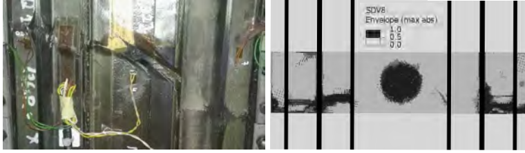
Fig. 6.15: a) Back - face image of the experimentally tested CAI panel and b) the numerical model.
