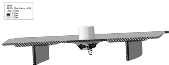
Fig. 6.12: View of impactor penetration through composite skin at instant u/u_{max} = 0.8 . Field output of the fiber damage variable (SDV8).
