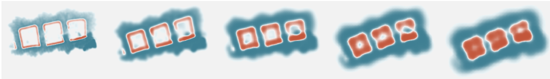
Figure 6.1: Comparison of different feature resolutions f_{res} while number of particles is 20 and the radius of the neighborhood is defined as r_{th} = 2f_{res} . From left to right, resolutions are 0.5, 1.0, 1.5, 2.0 and 2.5 m .
