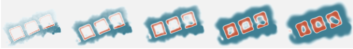
Figure 6.3: Comparison of different radius of neighborhood r_{th} while the feature resolution f_{res} is kept constant at 1 m resolution. From left to right, radius are 1.0, 1.5, 2.0, 3.0 and 4.0 m.
