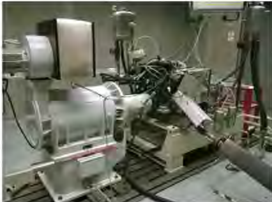
Fig. 7. Engine test bench. Engine Lab of Repsol Technology Center.
