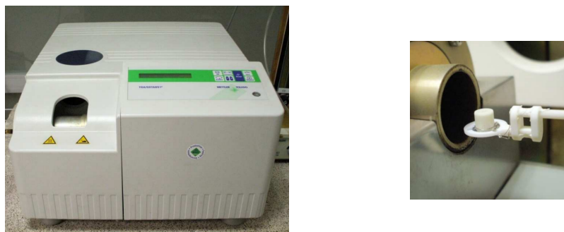
Fig. 3.11: Photograph of the Mettler-Toledo's TGA/SDTA851 used in this work and detail of the crucible support [146]
