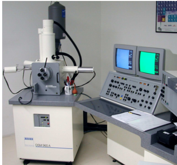
Fig. 3.4: The Zeiss DSM-960A microscopy used for the SEM characterizations [127]
