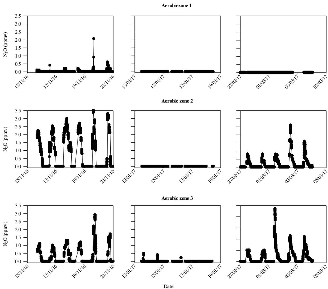
**Figure 7.2:** N<sub>2</sub>O emissions from aerobic zones 1, 2 and 3 of the plug-flow reactor in November (left), January (center) and March (right).
