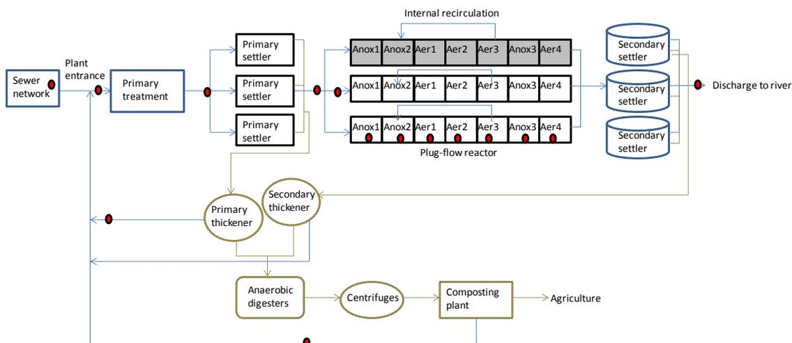
**Figure 3.4:** Scheme of the configuration of the WWTP of Girona (in grey is marked the plug-flow reactor line where the gas collection hoods were placed and the red dots represent the  $\text{CH}_4$  dissolved grab samples).
