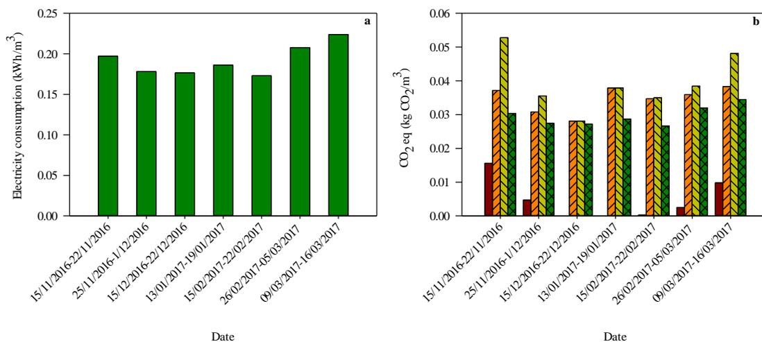
**Figure 7.6:** Electricity consumption (a) and direct (N<sub>2</sub>O, CH<sub>4</sub>) and total direct emissions (N<sub>2</sub>O + CH<sub>4</sub>) and indirect CO<sub>2</sub> emissions (indirect) (b) from the plug-flow reactor of the WWTP along the monitoring period.
