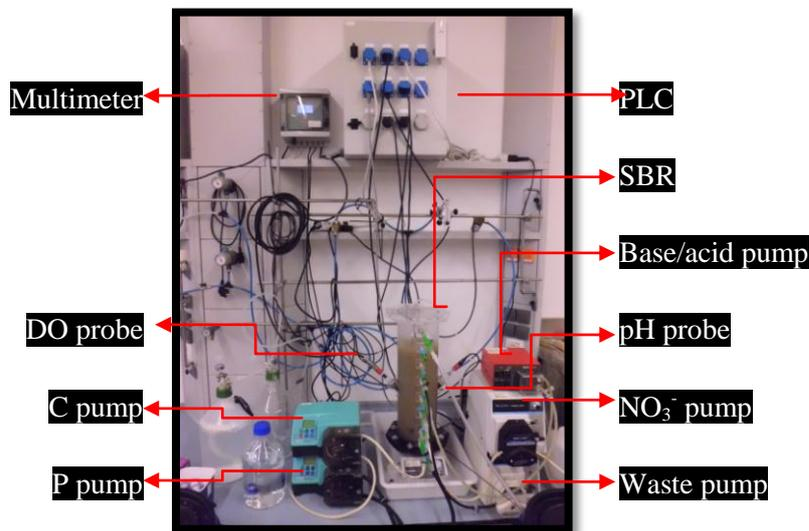
**Figure 3.2:** Typical SBR used at ICRA laboratories (the image in this case corresponds to the dGAO reactor).
