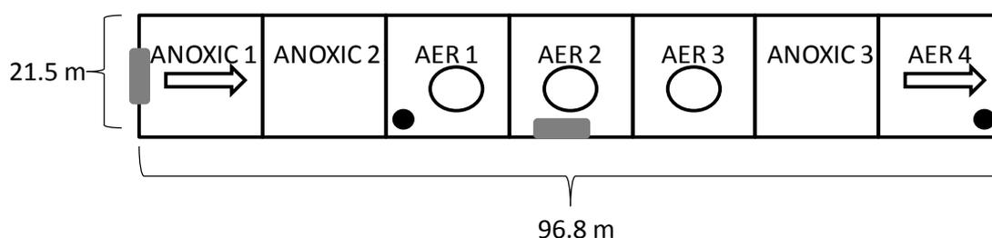
**Figure 7.1:** Plug-flow reactor configuration and zone of study. The black dots represent the plant DO sensors located in aeration zone 1 and aeration zone 4. The squares represent the online ammonia sensors at the inlet of the plug-flow reactor and in aeration zone 2. The white dots represent the place where the gas hoods were placed. The arrows represent the direction of the wastewater flow.
