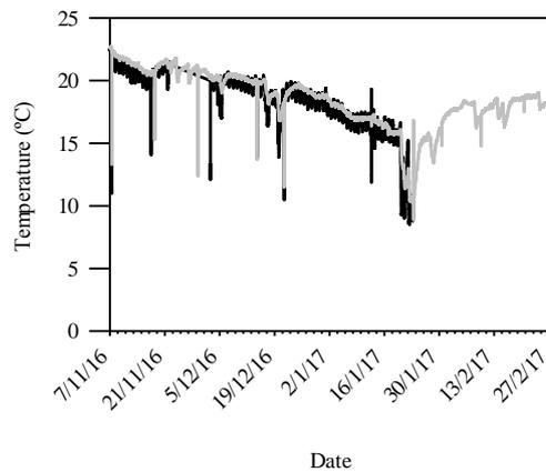
**Figure SI.5:** Profile of the temperature of the wastewater from November till late February of aeration zone 2 (—) and influent of the reactor (---).
