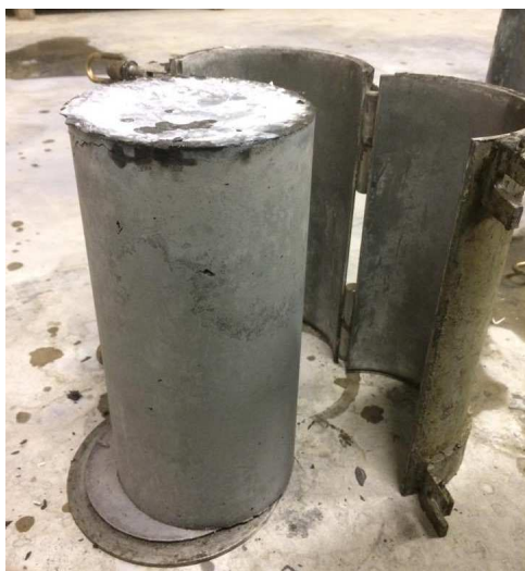
Figure 3.12: Demolding of the cylinders
