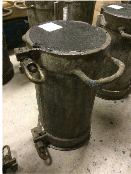
Figure 3.11: Cylindrical mold filled with UHPFRC
