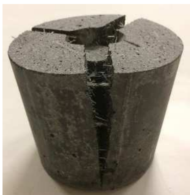
Figure 6.11: Crack more wide at the top than at the bottom
