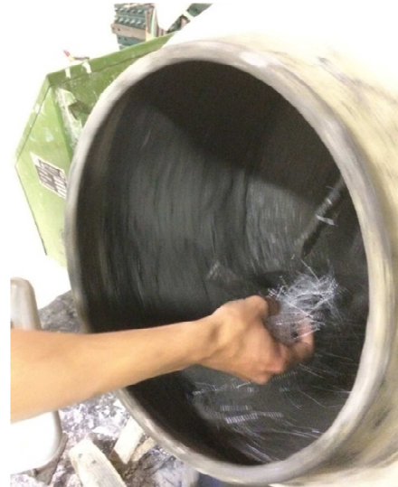
Figure 3.9: Addition of the fibres during mixing
