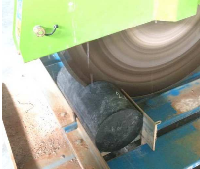
Figure 3.10: Cutting of cylinders giving two specimens
