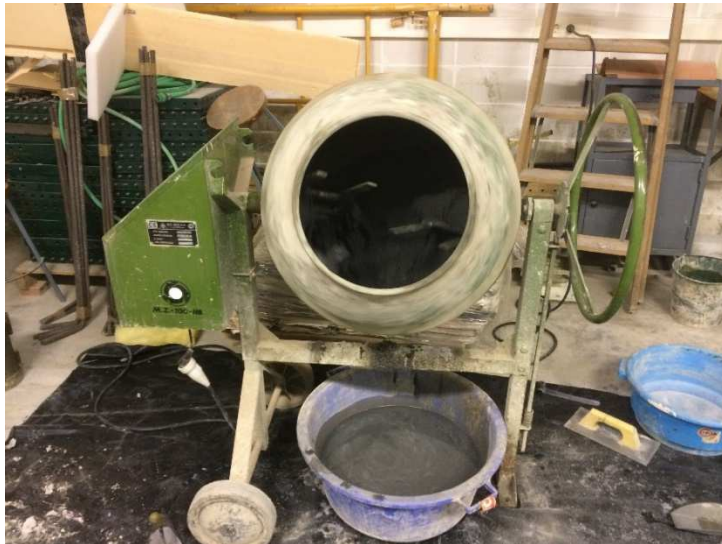
Figure 3.8: Drum mixer mixing UHPFRC
