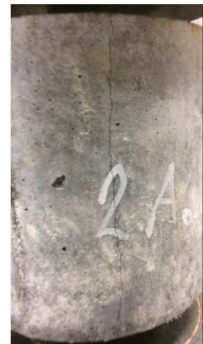
Figure 6.10: Crack equally wide across the entire height of the specimen
