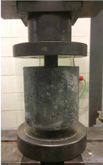
Figure 3.15: Specimen during Barcelona test
