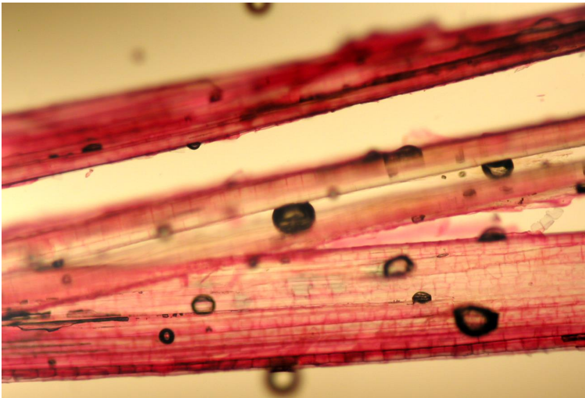
Figure 4-24: Flax fiber treated with XTI at 0.3 %, 40 °C and pH 5 during 24 hours augmented 40 times observed through a microscope.
