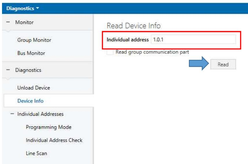
Figure 58 - ETS5 Device Info (read individual address)
