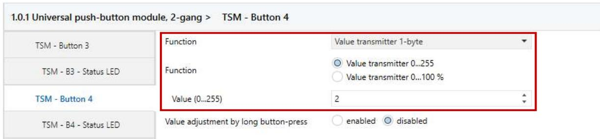
Figure 108 - ETS5 Universal push-button module (Button 4 value transmitter 1-byte)
