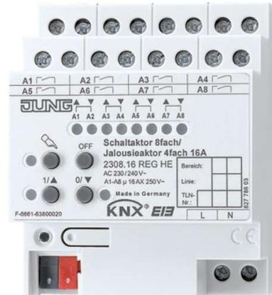
The switch/blind actuator receives telegrams from sensors or other controls via the KNX and switches electrical loads. The relay outputs can be set in ETS to blinds operation or to switching operation. Mixed operation is also possible.
