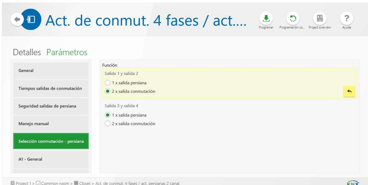
**Figure 86 - ETS Inside (Parameters of the switching actuator)**
