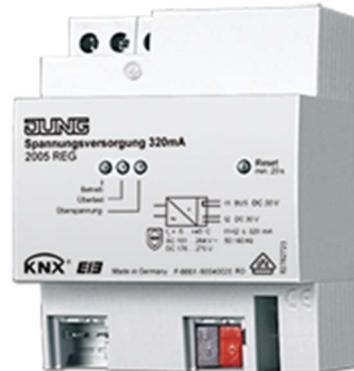
The power supply 320 mA produces and controls the system power for the KNX. The devices can be connected to a bus line via the terminal BUS, without an additional choke. Furthermore, the power supply offers a 30 V DC output to supply a further bus line (i.e. main line). For this an additional choke is required.
