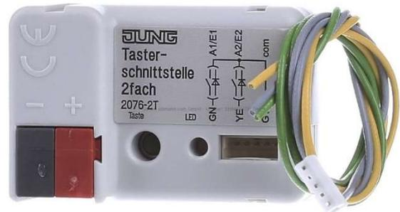
The 2-channel push-button interface has 2 independent channels which can be used as an inputs or alternatively as outputs. The push-button interface can therefore be used to poll its inputs for the switching state of up to 2 potential-free push-buttons/switches with a common reference potential and send the corresponding telegrams to the KNX.
