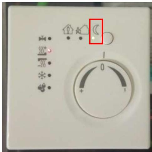
Figure 112 - KNX Room temperature controller (Night mode)
