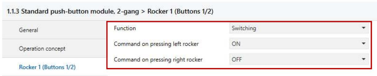
Figure 99 - ETS5 Standard push button (Rocker 1)
