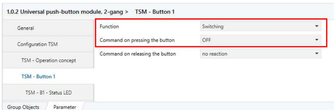
**Figure 35 - ETS5 Universal push-button module (Button 1 switching OFF)**
