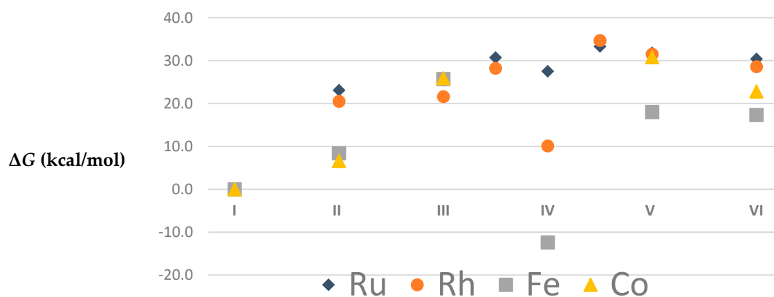
Figure 1. Reaction pathway (BP86-D3BJ/TZVP~sdd//BP86-D3BJ/TZVP~sdd Gibbs free energies in solvent in kcal/mol) for the olefin metathesis reaction pathway for M(\text{SIMes})\text{Cl}_2(=\text{CHPh})\text{PPh}_3 ( M = \text{Ru} and \text{Rh} ) with ethylene as substrate.
