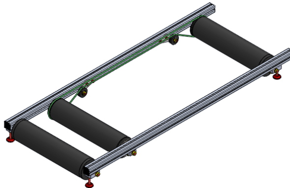
Figura 3. Estructura principal, 1400x580x145mm
