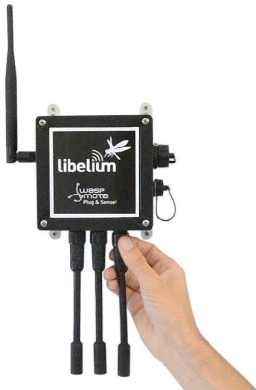
Figure : Connecting a sensor probe to Wasmote Plug & Sense!
