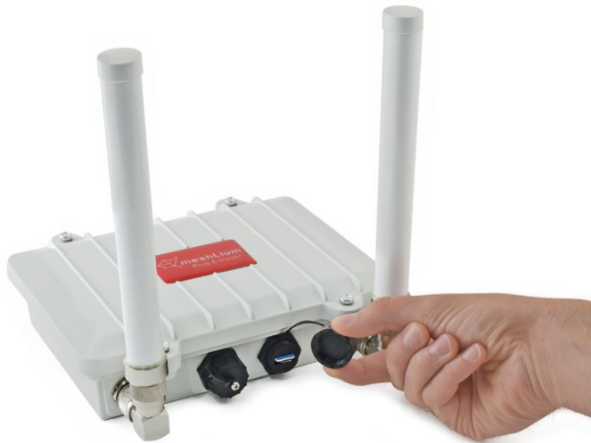
Figure : External SIM socket in a Meshlium with 3G/GPRS module
