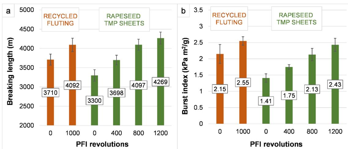
Fig. 4. Effect of refining in the breaking length and burst index of isotropic sheets from commercial fluting and from rapeseed stalk high-yield pulp.
