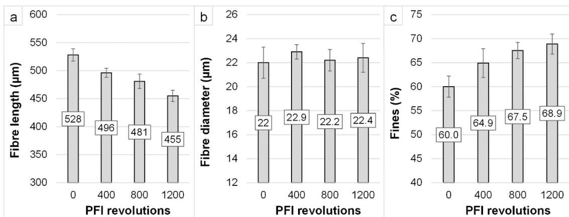
**Fig. 3.** Effect of refining on the average fibre length (a), on the average fibre width (b) and on the percentage of fines (c) in the thermomechanical pulp
