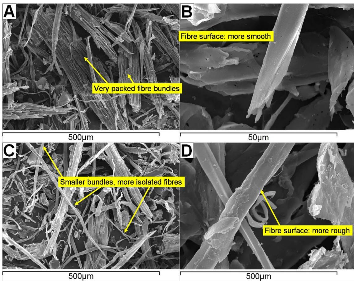
**Fig. 2.** SEM images of the mechanical pulp from rapeseed stalks with a magnification of 100 (a) and 1000 (b), and of the thermomechanical pulp with a magnification of 100 (c) and 1000 (b)
