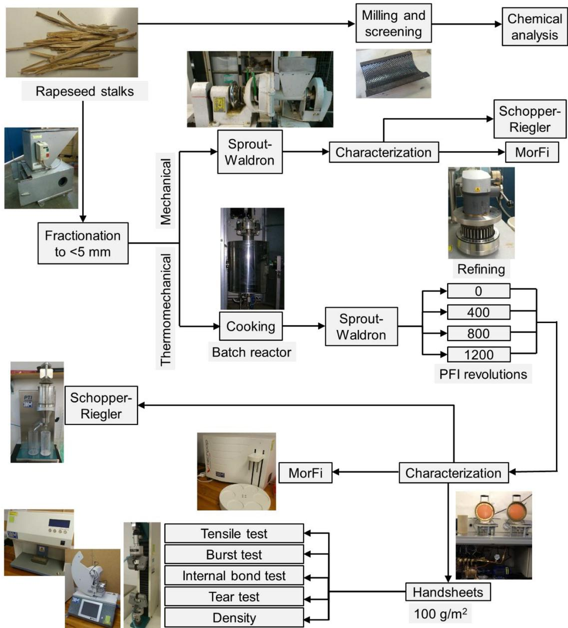
Fig. 1. Experimental procedure regarding the mechanical and thermomechanical pulp
