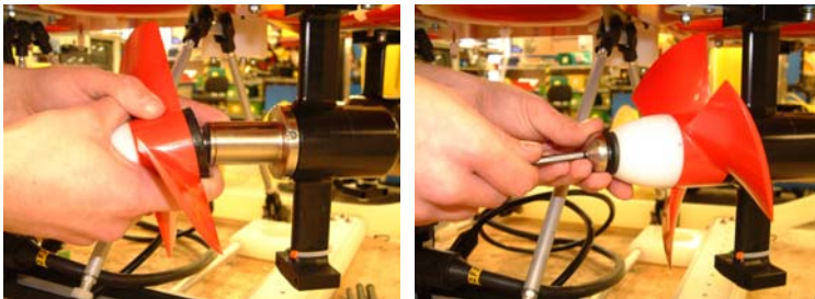
Fig. 11. Thruster Propeller Fitment
