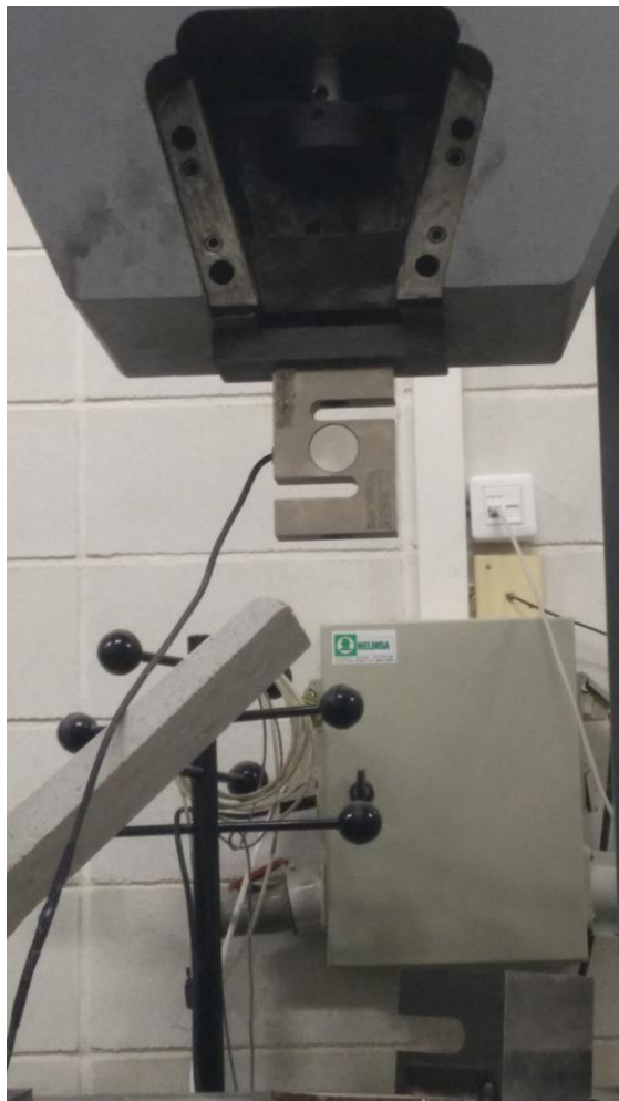
Figure 4.12 Attaching load cell
