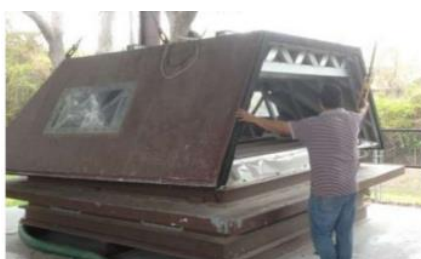
Figure 4.1 UL 580 , uplift test
