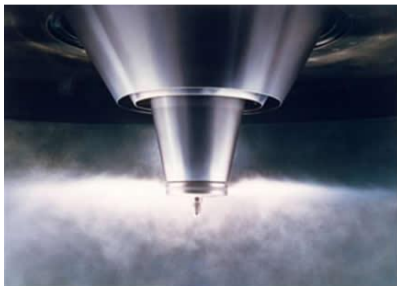
Spray Drying Technology: rotary atomizer in a spray dryer
