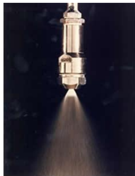
Spray Drying Technology: nozzle atomizer in a spray dryer
