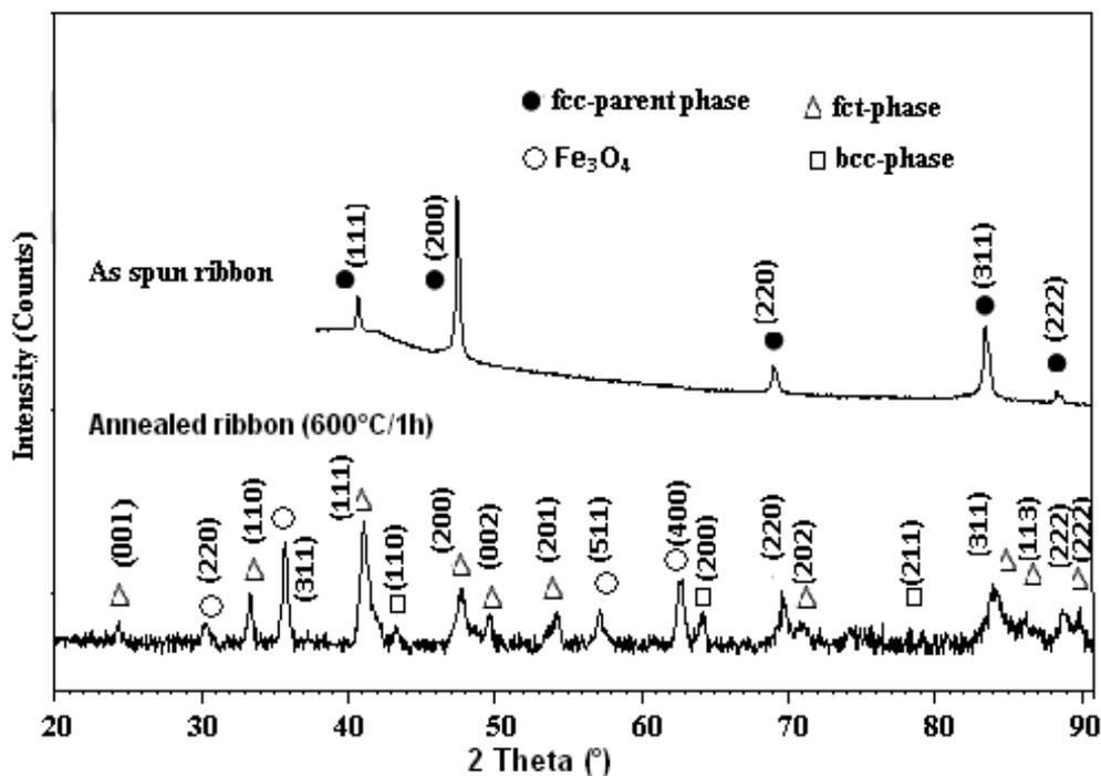
**Figure 2.** XRD patterns of as-spun and annealed  $\text{Fe}_{68.45}\text{Pd}_{28.21}\text{Co}_{1.66}\text{Ni}_{1.66}$  ribbons.
