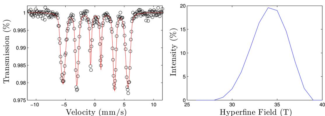
**Figure 4.** Collected Mössbauer spectra (**left**) with the experimental data (symbols) and the best fit (red line) and hyperfine magnetic fields distribution (**right**).
