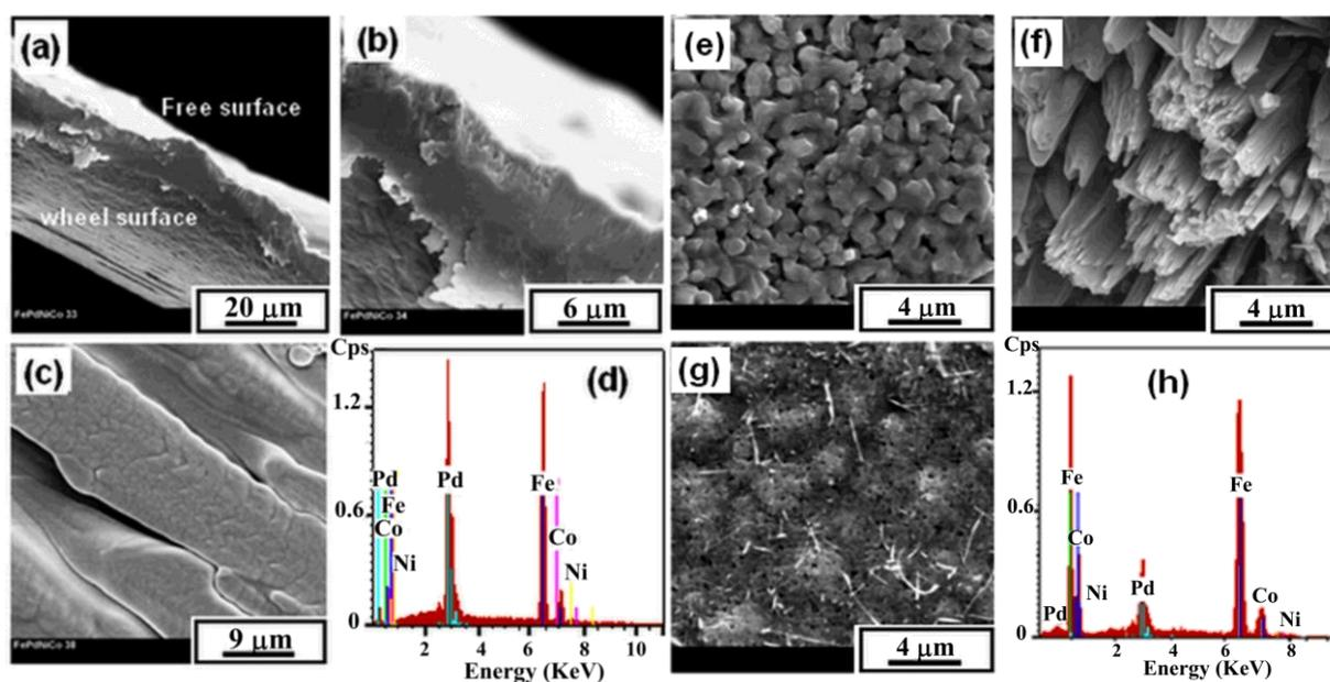
**Figure 1.** SEM micrographs of microstructure exhibited by as-spun and annealed  $\text{Fe}_{68.45}\text{Pd}_{28.21}\text{Co}_{1.66}\text{Ni}_{1.66}$  ribbons at 600 °C for 1 h: (a) typical cross section; (b) higher magnification of cross section; (c) free surface for as-spun ribbons; (d) EDX corresponding to the as-spun ribbons; (e) free surface for annealed ribbons; (f) View of microwires growth; (g) wheel surface for annealed ribbons and (h) EDX corresponding to the annealed ribbons.
