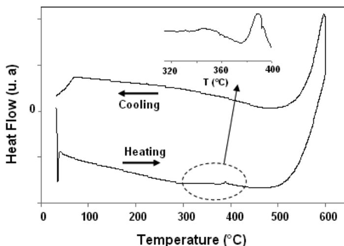
**Figure 3.** DSC scans for as-spun ribbons upon heating and cooling at a rate of 10 K/min.
