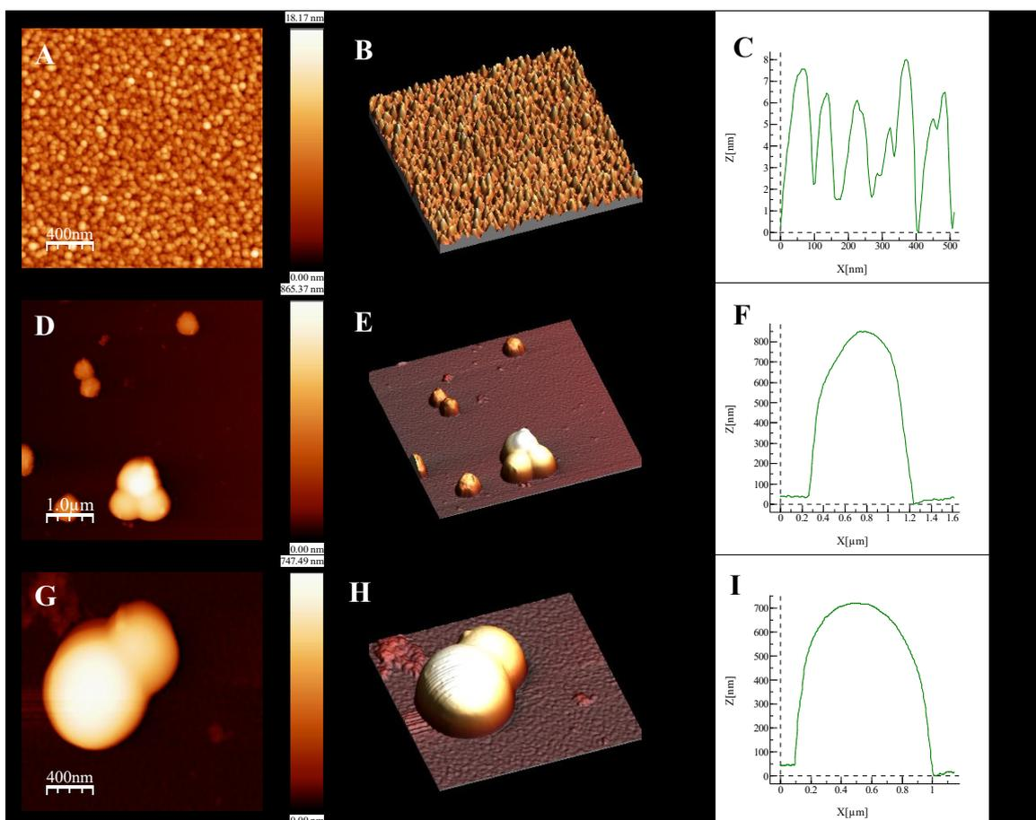
**Figure 12.** AFM results. Each row displays three pictures: first one is a topography picture, second one is its 3D representation and last one shows the respective topography profile of each surface. First row displays bare gold surface results. Second row is a maleimide *L. lactis* IB-incubated substrate showing their adhesion to the SAM. Third row is a closer look to IBs.
