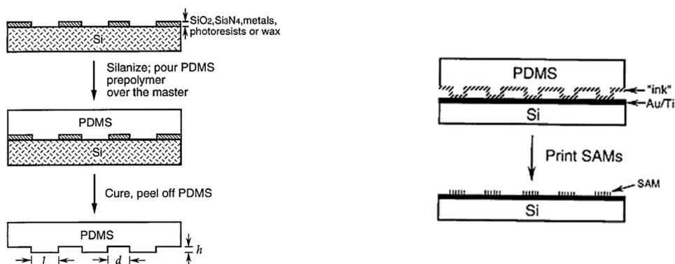
**Figure 6.** Left : preparation of PDMS stamp pouring PDMS to a patterned master, curing and peeling. Right : microcontact printing of SAMs using PDMS stamp [19].
