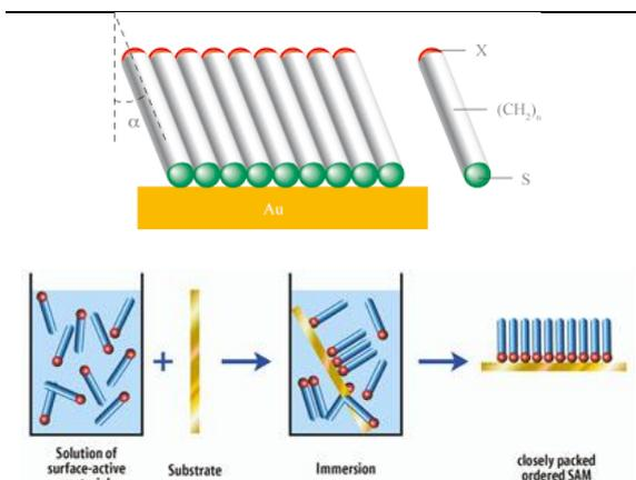
**Figure 1.** Top image shows a SAM disposed on a gold substrate [4]. Red color represents the terminal group, white is the spacer chain and green shows the head group. Second scheme shows the SAM spontaneous self-organization [5].
