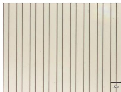
**Figure 10.** Microscope picture of the PDMS microcontact printing stamp pattern used in this study.
