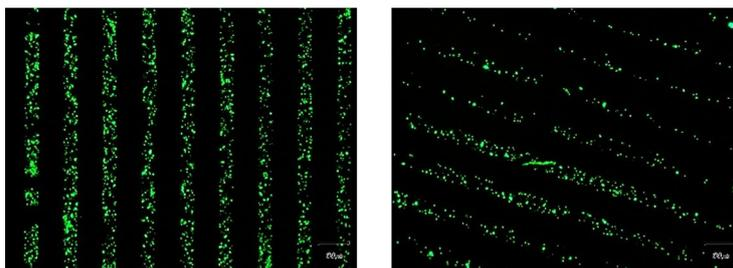
**Figure 17.** Representative fluorescent microscopy images of  $20\mu\text{m}$  striped  $\mu\text{CP}$  patterns of GFP IBs on prefucionalized surfaces. Left: *E. coli* IB patterns. Right: *L. lactis* IB stripes. *L. lactis* pattern displays poorer adhesion compared to the *E. coli* IBs substrate. Scale bar indicates  $30\mu\text{m}$ .
