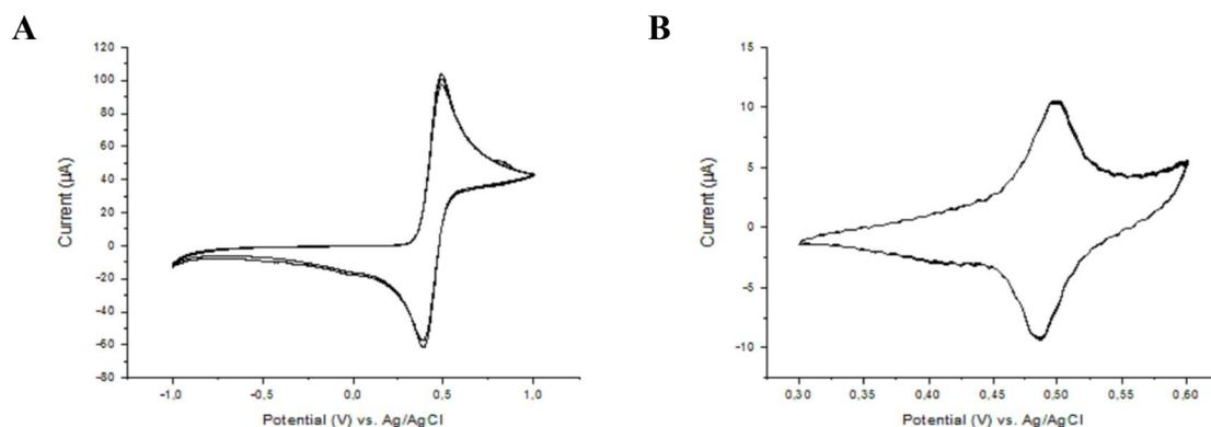
**Figure 16.** A: cyclic voltammetry of ferrocene in solution. B: maleimide-ferrocene SAM was used as the working electrode.
