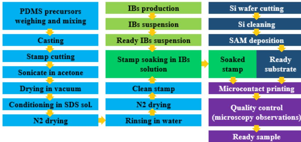
**Figure 11.** Overall flow chart of the two-dimensional microscale structuration of IBs on surfaces. Each block represents an operation and arrows visualize the flow direction. Operations regarding PDMS stamp, IBs suspension, silicon substrate and  $\mu$ CP sample are marked in light blue, green, blue and purple, respectively [22].
