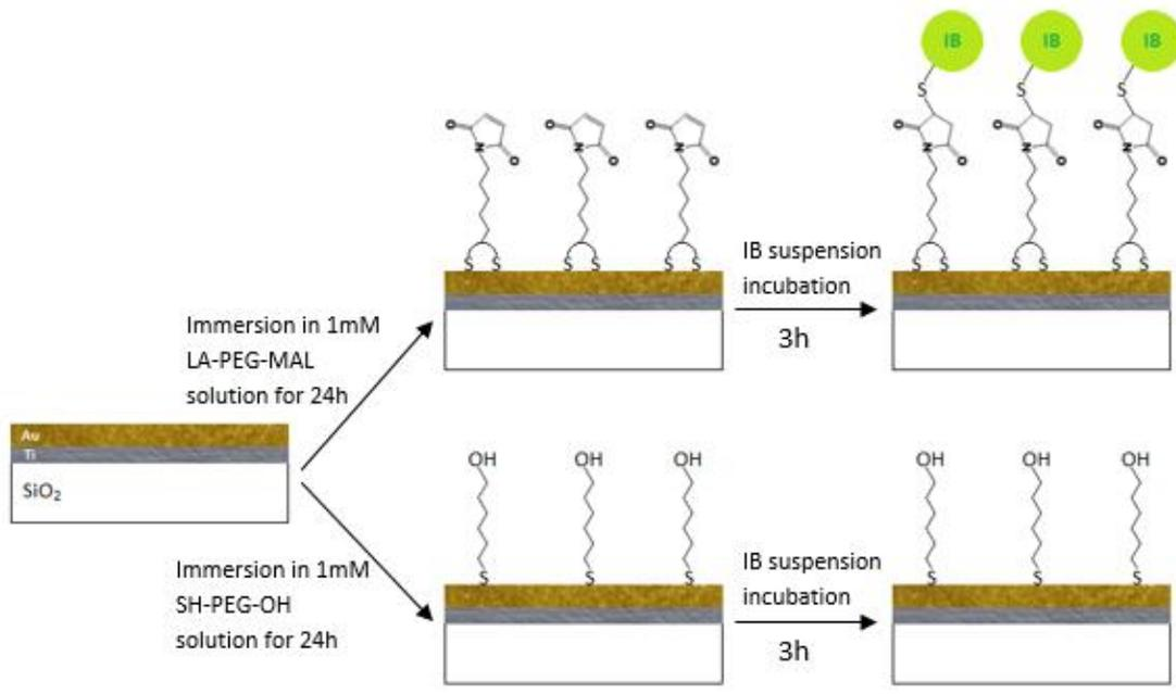
**Figure 9.** Scheme of the study of IB interaction with maleimide. At first, titanium and gold will be deposited by evaporation on SiO<sub>2</sub> wafers. Next step will be the functionalization with LA-PEG-MAL and SH-PEG-OH and finally IBs will be incubated on the surfaces. No IB adhesion is expected on SH-PEG-OH SAMs and covalent IB adhesion to maleimide SAMs is predicted.
