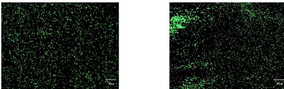
**Figure 13.** Fluorescence microscopy images of SH-PEG-OH SAM after IB incubation with PBS at pH=7,59. Left picture was taken before intense rinsing and right picture immediately after the rinsing. No fluorescence loss is detected.
