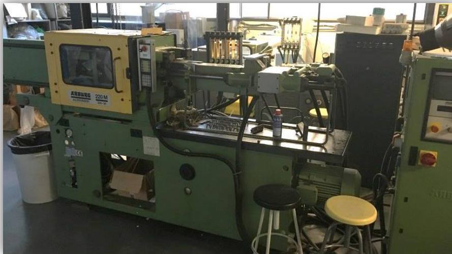
Figura 3.12 Injectora Arburg model Allrounder 220M
