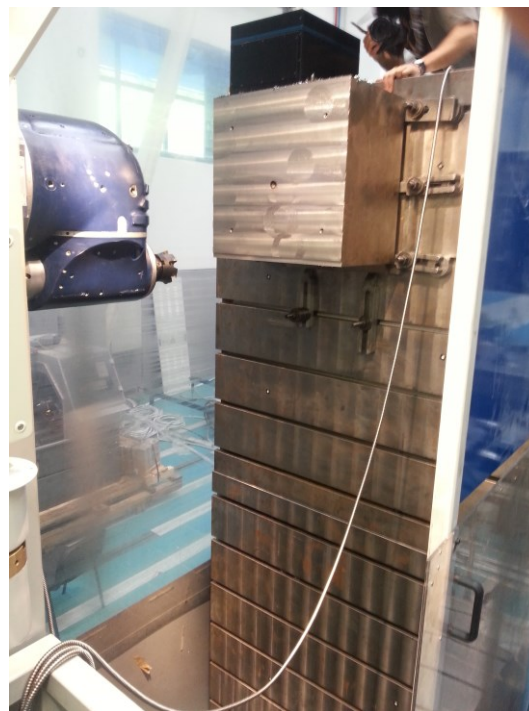
Figure 10.14: Experimental setup of VSTMD on FXR machine.
