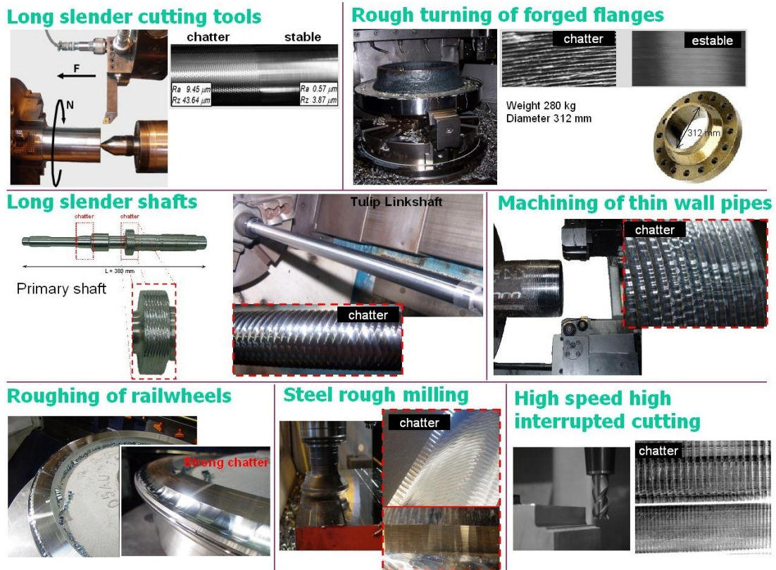
Figure 2.4: Typical operations in which chatter may occur.
