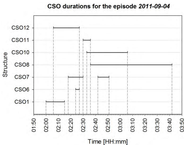
**Figure 4-1-6.** Duration of the CSOs produced at different structures for a 2.50 mm rainfall episode occurred on 04/09/2011. Horizontal black lines indicate the starting and ending point of CSO for each structure. It can be observed that CSO1, 12 and 7 are the ones overflowing at the beginning and that a consecutive activation/deactivation of all the overflows occurs. The structures that do not appear means that no CSO was produced for such structures.
