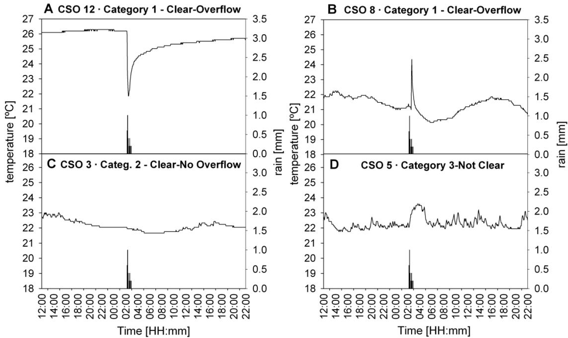
**Figure 4-1-3.** Different categories of temperature responses used to evaluate the method effectiveness. Black lines represent the temperature profiles. Vertical black bars represent the rainfall data. The four subplots correspond to the same time rainfall episode, from 04/09/2011. From A to D: *Category 1 – Clear-Overflow negative*, *Category 1 – Clear-Overflow positive*, *Category 2 – Clear-No Overflow* and *Category 3 – Not Clear* response.
