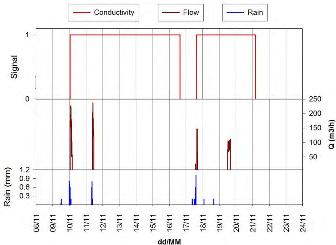
**Figure AIII-3.** Monitoring period from 08 to 24 November 2012 in the CSO Structure 14 (CSS of La Garriga). Four CSO events were detected with the flowmeter. The conductivity sensor only detected two events because of solids attached on the sensor, which produced a prolongation of the conductivity signal.
