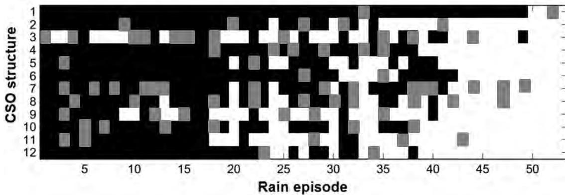
**Figure 4-2-7.** A plot of the predicted and observed responses of each CSO structure for 53 rain episodes that occurred in La Garriga. The black squares indicate instances where the model correctly predicted overflow (the prediction matched observation), the white squares indicate when the model correctly predicted that an overflow did not occur, and the grey squares show where the model incorrectly predicted overflow or no overflow (the prediction did not match observation).
