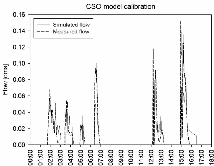
**Figure AV-1.** Simulated and measured flow profiles from the CSO structure calibration.
