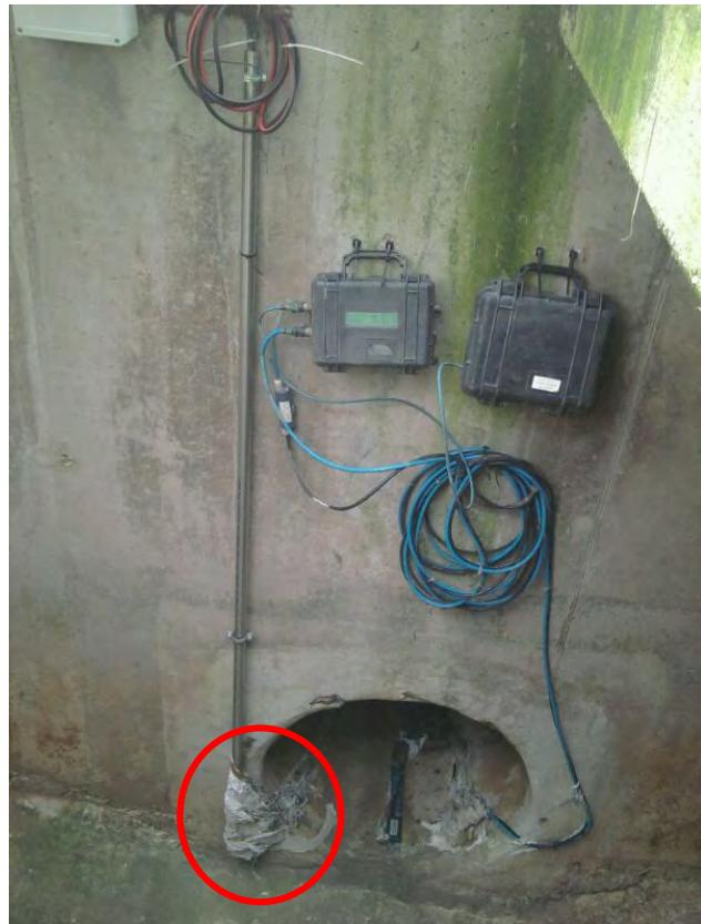
**Figure AIII-4.** Solids attached on the conductivity sensor (16-Nov-2012).
