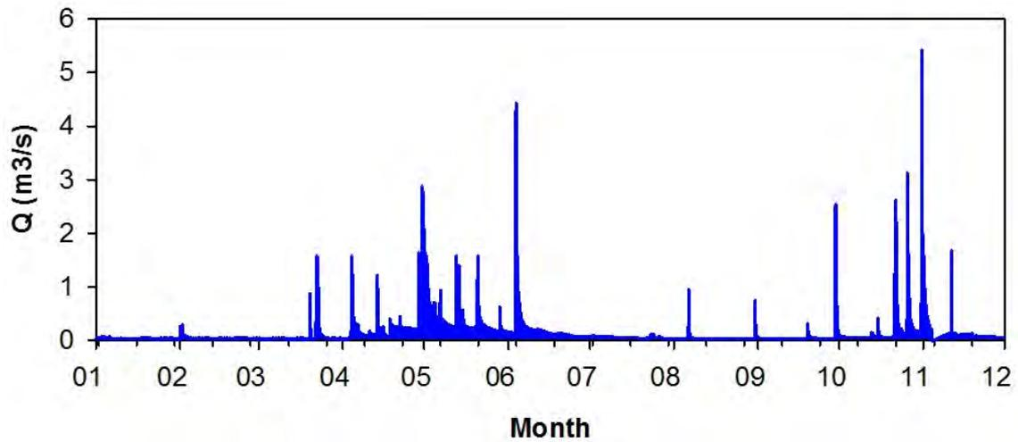
**Figure 3-5.** Flow discharge rate (in m<sup>3</sup>/s) for the year 2012, measured by a gauging station in the Congost River.
