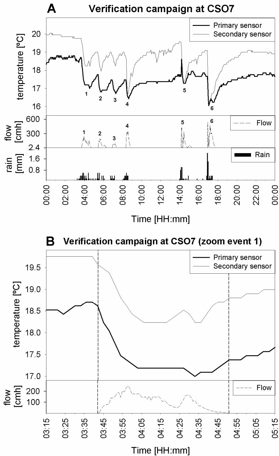
**Figure 4-1-2.** Temperature and overflow profiles from the method verification campaign. [A] plots temperature, flow and rainfall data from the verification period, representing 6 overflow events (numbered) within 24 hours, each CSO event corresponding to a temperature shift. [B] is a zoom of event 1 in which vertical dashed lines indicate the start and end points of the CSO event.
