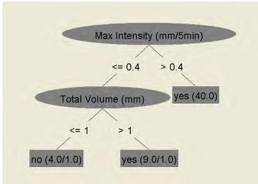
**Figure AVII-1.** Decision tree constructed for the CSO Structure 14.**“La Garriga CSO Network Simulator”**
