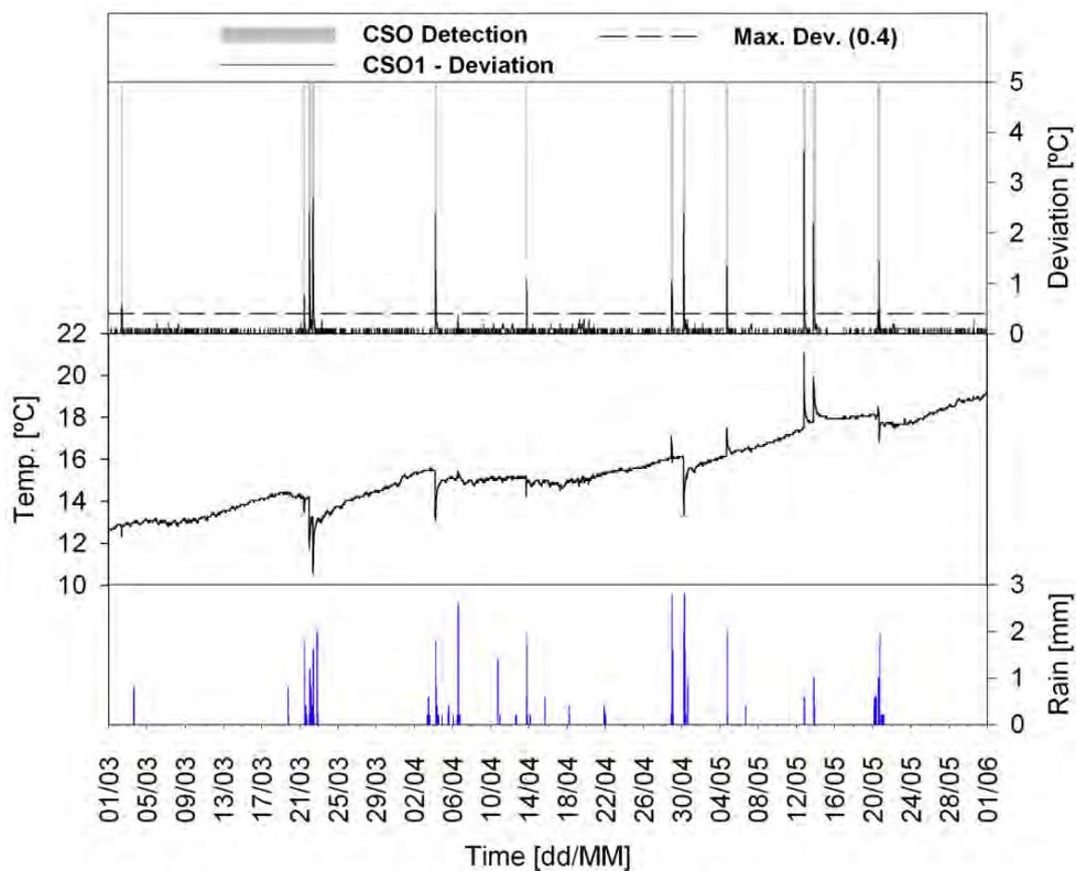
**Figure 4-1-7.** Automatic detection of CSO events for the structure CSO1 for the period from [01-03-2012] to [01-06-2012]. A window length of 60 min and predefined maximum deviation of 0.4 °C were selected. On the top part, vertical grey bars indicate the automatic detection of the CSOs, matching with the temperature shifts below.
