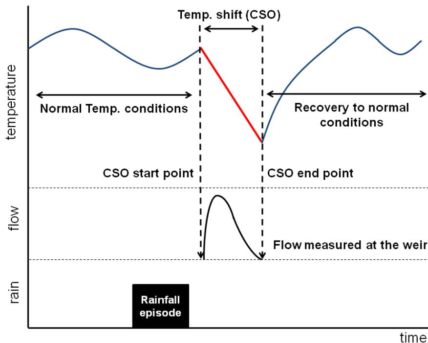
**Figure 4-1-1.** Theoretical graph representing the principle of the CSO detection method.
