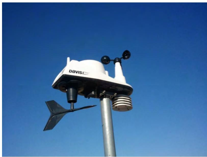
**Figure 3-11.** Weather station installed on the rooftop of the La Garriga city Council.
