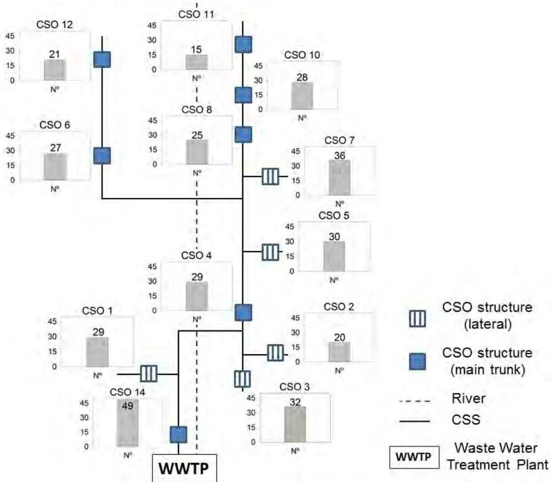
**Figure 4-2-6.** Schematic of the La Garriga CSS. The number of overflows that occurred in each CSO structure during the 11-month study is graphed.
