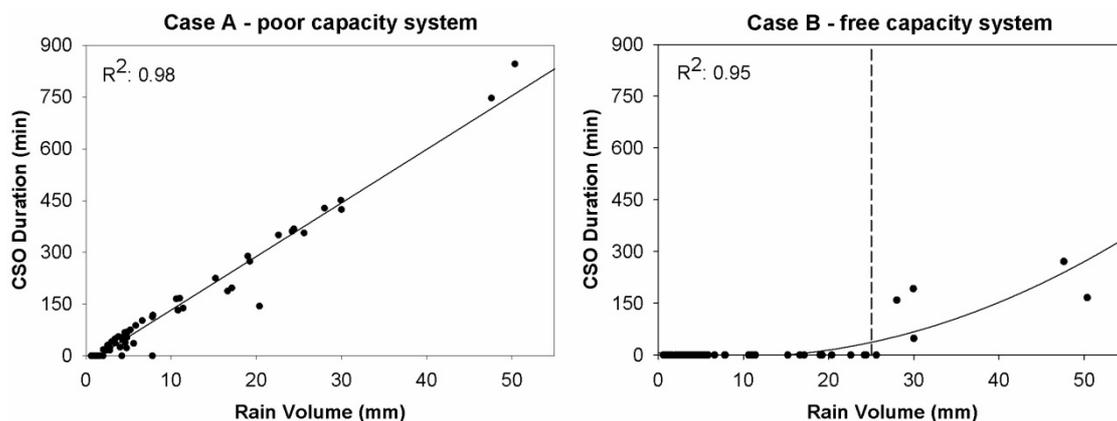
**Figure 4-2-1.** CSO duration versus rain volume for two hypothetical CSSs. Case A shows data from a CSS with high CSO activity, while case B shows data from a system with higher capacity. In case B, the vertical dashed line indicates approximately the maximum volume of rain (about 25 mm) that the system can assimilate before it begins to overflow.
