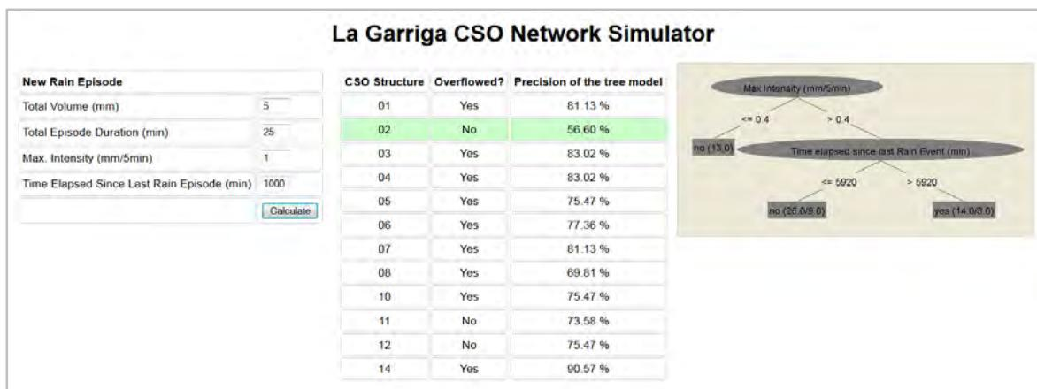
**Figure AVII-2.** The *La Garriga CSO Network Simulator* interface, with an example of the overflow predictions made for a rain episode with user-input characteristics; an overflow prediction is made for each CSO structure (with CSO structure 2 highlighted and its tree shown in the image).
