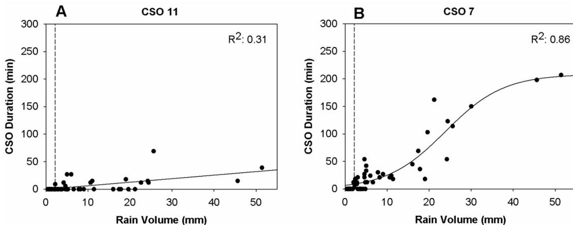
**Figure 4-2-2.** Rain volume versus overflow duration obtained for CSO Structures 11 and 7 during the studied period (53 rain episodes). The vertical dashed line indicates approximately the maximum rain volume that the system can assimilate before it begins to overflow, which was 2.2 mm in both cases.
