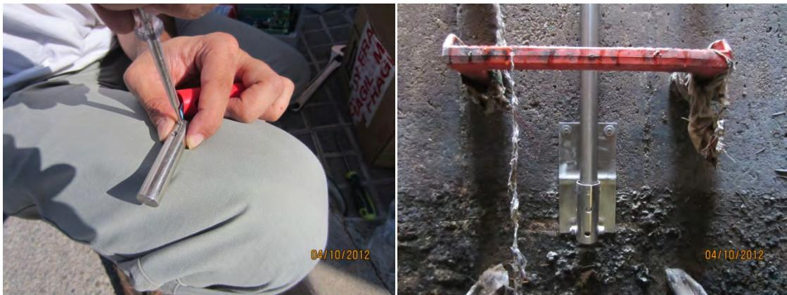
**Figure 3-12.** On the left, detail of the conductivity sensor. On the right, detail of the mounting accessory (with the sensor inside).
