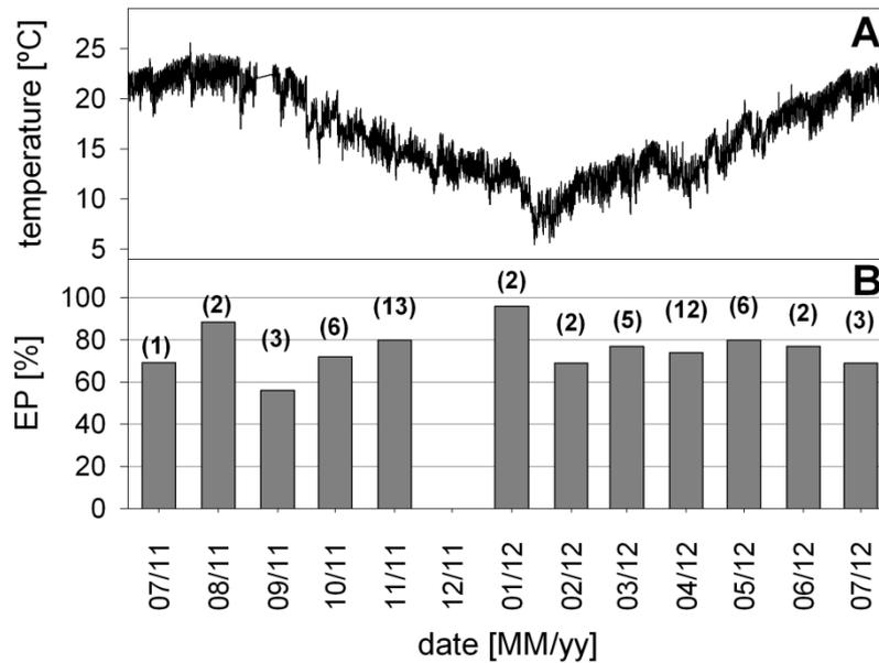
**Figure 4-1-5.** Seasonal variation of temperature. [A] shows the temperature profile registered at the structure CSO6 from July 2011 to July 2012. [B] shows the calculated monthly expected potential rates (EP's) averaging for all the structures. In parenthesis the number of rainfall episodes per month is indicated. Note that in December 2012 there is no bar chart because there were no rainfall episodes.
