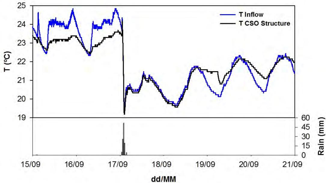
**Figure AIII-1.** Prolonged temperature convergence after the CSO event due to solids attached on the sensor in the inflow channel.
