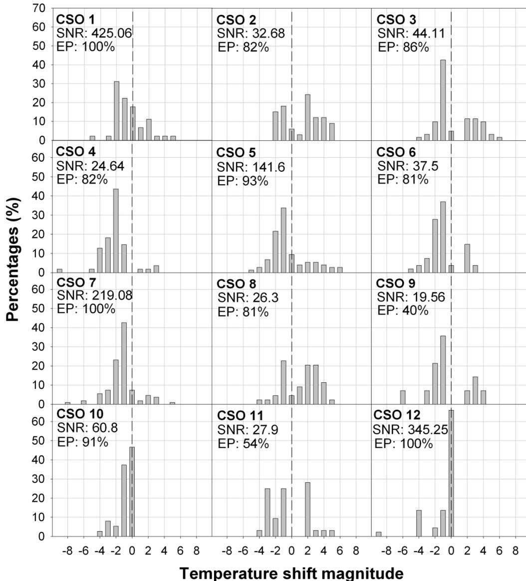
**Figure 4-1-4.** Percentage distribution of the temperature shift magnitudes for each CSO structure for all the period of study. The vertical black dashed line in each histogram marks the 0 °C shift magnitude (grouping changes from 0 to  $\pm 1$  °C). For each structure the SNR and the EP are presented. Note that the structure CSO13 (SNR-28.09) is not represented due to the very low number of *Clear* responses.
