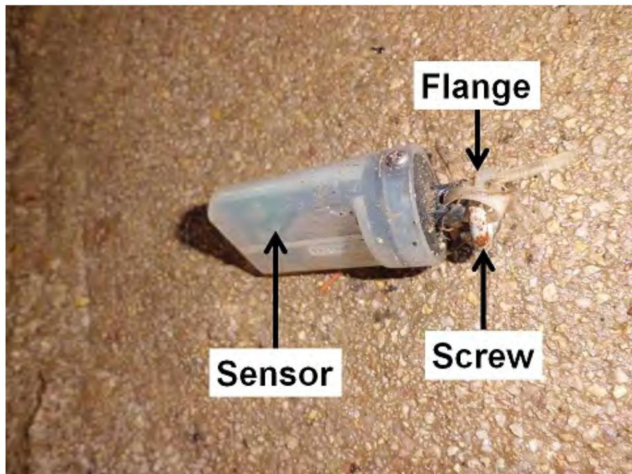
**Figure AI-1.** Detail of the sensor attachment to the CSO structure.
