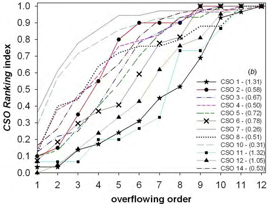
**Figure 4-2-5.** Ranking curves for each CSO structure. The y-axis is the ranking index, and the x-axis is the  $i^{\text{th}}$  place of overflow in the network. In the legend shows in parentheses the value of exponent  $b$  of the power function fitted to each curve.
