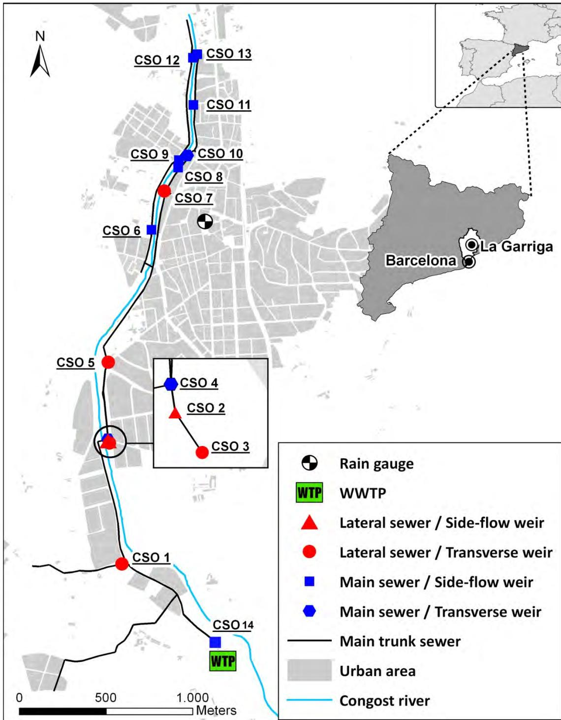
**Figure 3-6.** Overview of the urban wastewater system of La Garriga (Montserrat et al., 2013).
