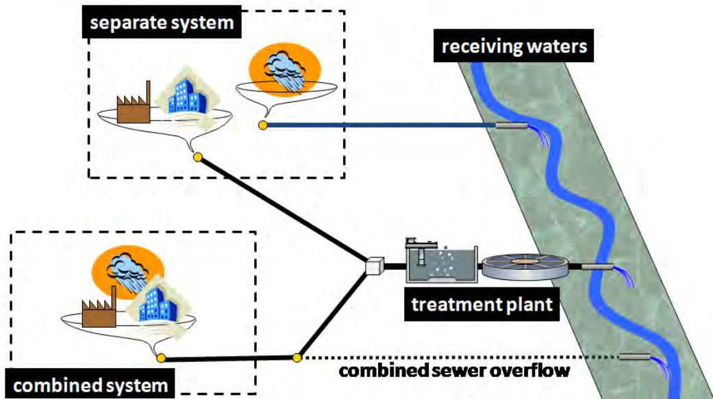
**Figure 1-1.** Conceptual scheme of an urban wastewater system (adapted from Devesa, 2006).
