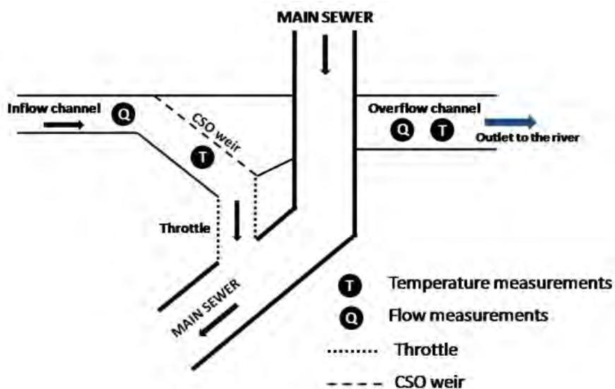
**Figure 3-9.** Layout and instrumentation of the monitoring station at the CSO structure of the Graz West Catchment.
