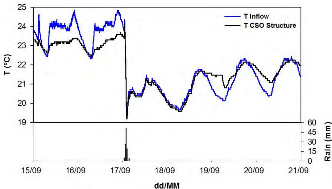
**Figure AIII-1.** Prolonged temperature convergence after the CSO event due to solids attached on the sensor in the inflow channel.
