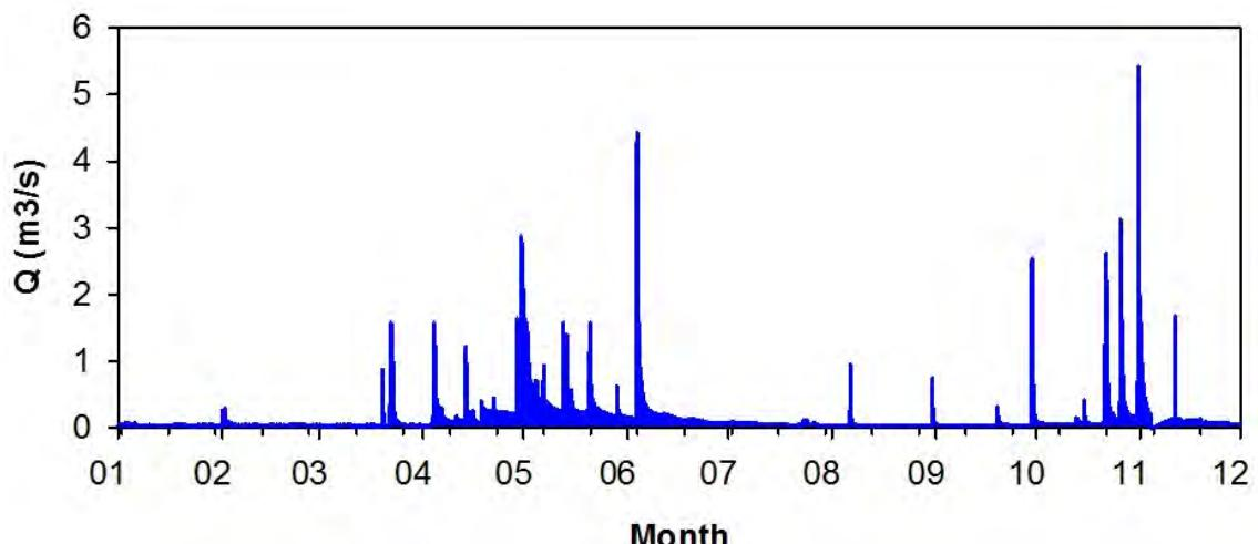
**Figure 3-5.** Flow discharge rate (in  $m^3/s$ ) for the year 2012, measured by a gauging station in the Congost River.
