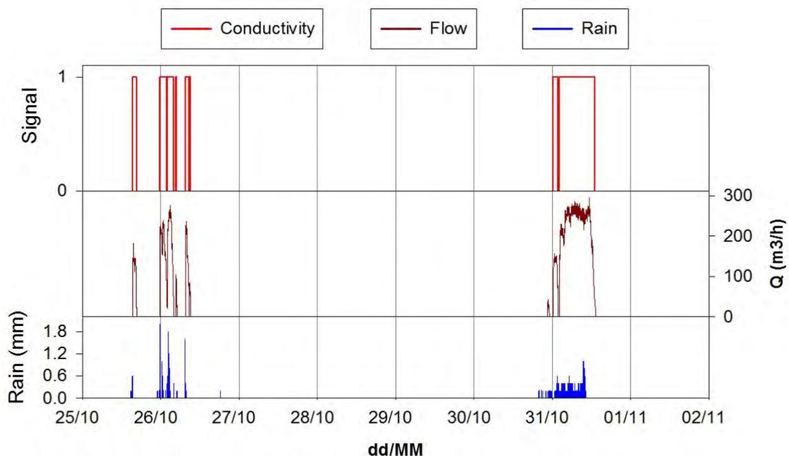
**Figure 4-1-9.** Monitoring period from 25-Oct to 02-Nov 2012 in the CSO Structure 14 from the CSS of La Garriga. The start and end point of the conductivity signal coincide with the flow measurements.
