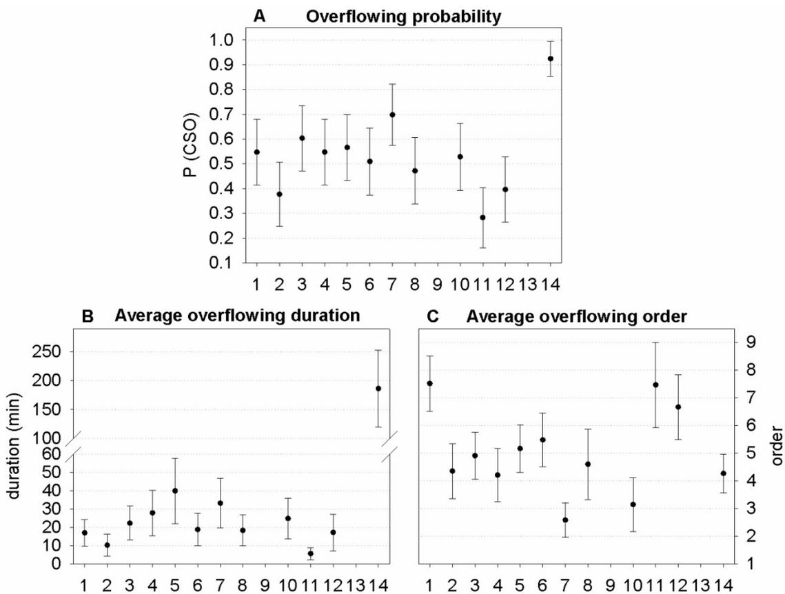
**Figure 4-2-4.** Evaluated parameters of the CSO structures (dots represent the average value, and the lines represent the 95% *Ci*). The x-axis is each structure of the CSS (note that Structures 9 and 13 do not have values because they were not used in this study).
