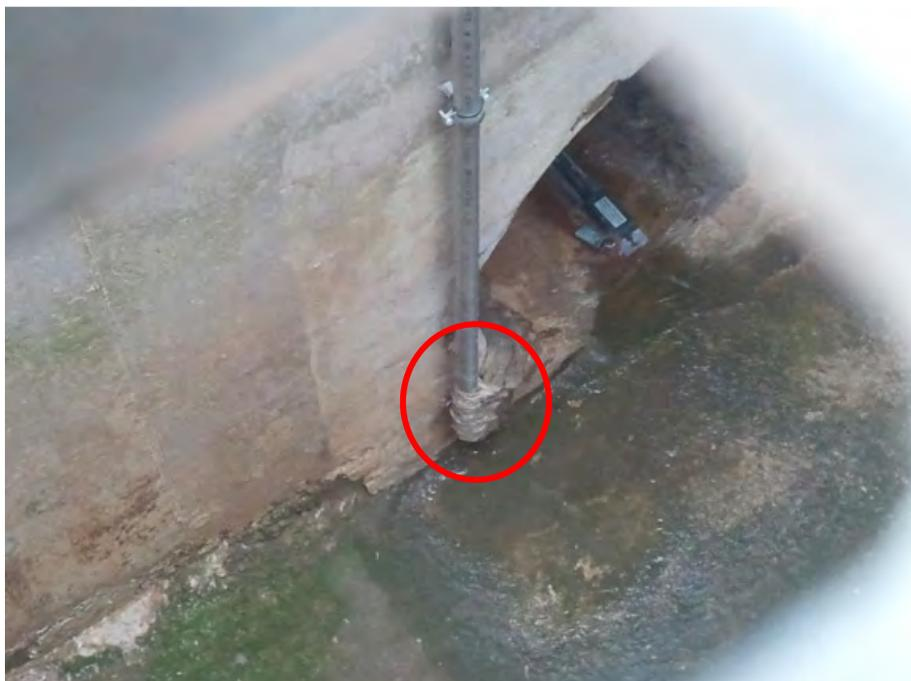
**Figure AIII-5.** Solids attached on the conductivity sensor (21-Nov-2012).
