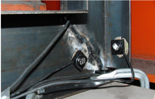
Figure 4.9 Placement of the accelerometers in the L-shape measuring device.
