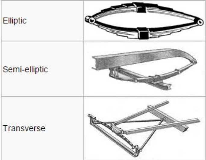
Figure 3.3 Different types of leaf springs designs.
