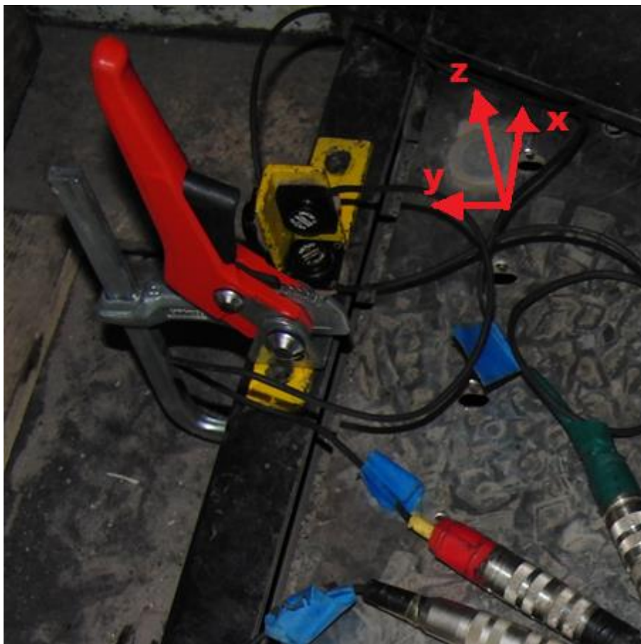
Figure 4.11 Accelerometers positioning inside the cabin for the recording of translation movements.
