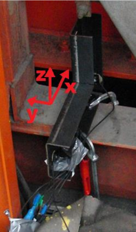
Figure 4.8 L-shape measuring device in position at the second crane measurement.
