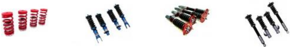
Figure 3.1 Different types of coilovers from left to right: Coilover sleeves, Non shock adjustable coilovers, Shock adjustable coilovers and Shock adjustable coilovers with camber kit.
