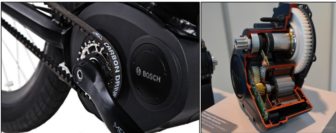
Figura 3. Motor central ( http://www.bosch-ebike.de )
