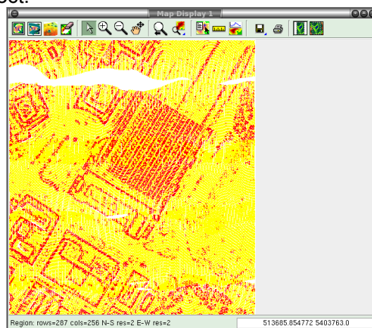
Figure 3: v.lidar.edgedetection output. Yellow: 'Terrain' points; Red: 'Edge' points.
