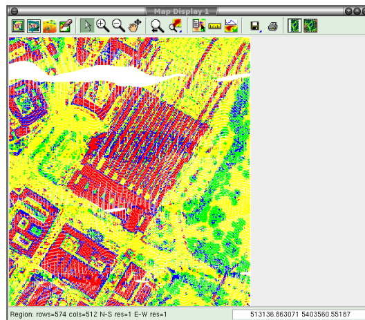
Figure 4: v.lidar.growing output. Yellow: 'Terrain single pulse' points; Green: 'Terrain double pulse' points; Blue: 'Object single pulse' points; Yellow: 'Object double pulse' points.
