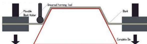
FIGURA 9. Two Point Incremental Forming with Complete Positive Die
