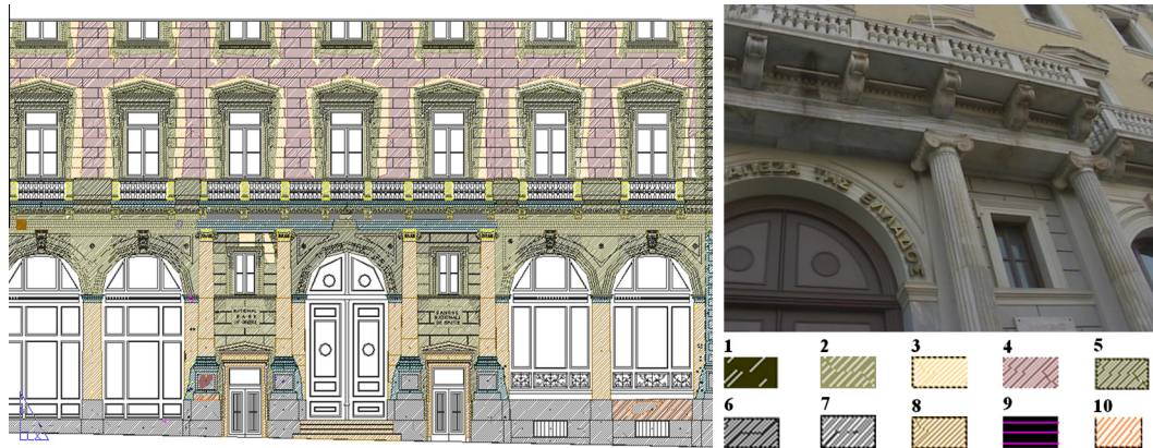
Fig. 18. CAD Mapping of decay patterns at the Mela Palace (north façade) [67].
