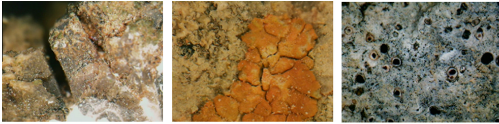
Fig. 13. FOM (50 \times ) at Erimokastro. Left: surfacial cracks on the dark-brown inclusion. Middle: Lichen on the off-white limestone. Right: carpic structure at the off-white limestone [66]. (For interpretation of the references to colour in this figure legend, the reader is referred to the web version of this article.)
