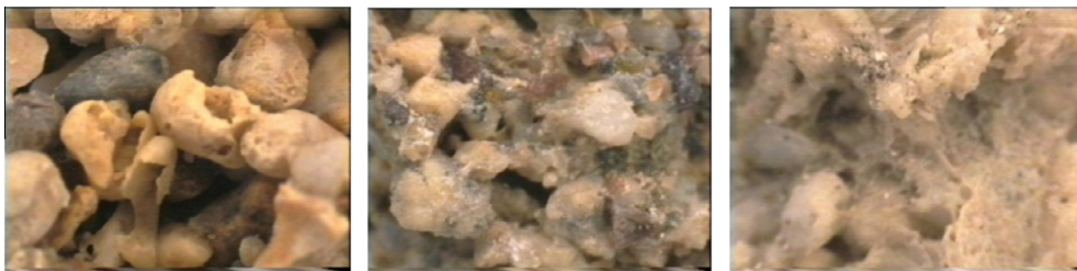
Fig. 15. Evaluation of consolidation interventions with FOM (50 \times ), Medieval City of Rhodes. Comparative microstructures of untreated porous stone (left), porous stone treated with a prehydrolyzed ethyl silicate with amorphous silica (middle), and porous stone treated with an aqueous colloidal dispersion of silica particles (right) [8,55].
