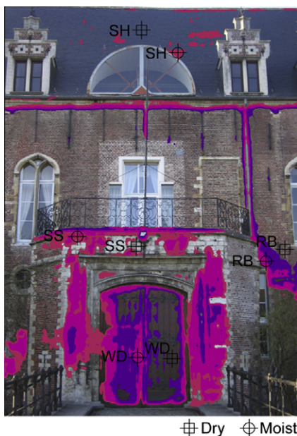
Fig. 13. Identified moist areas superimposed to the RGB image. Sample points are depicted as squared (dry areas) or crossed circles (moist areas). Naming corresponds to the considered material.
