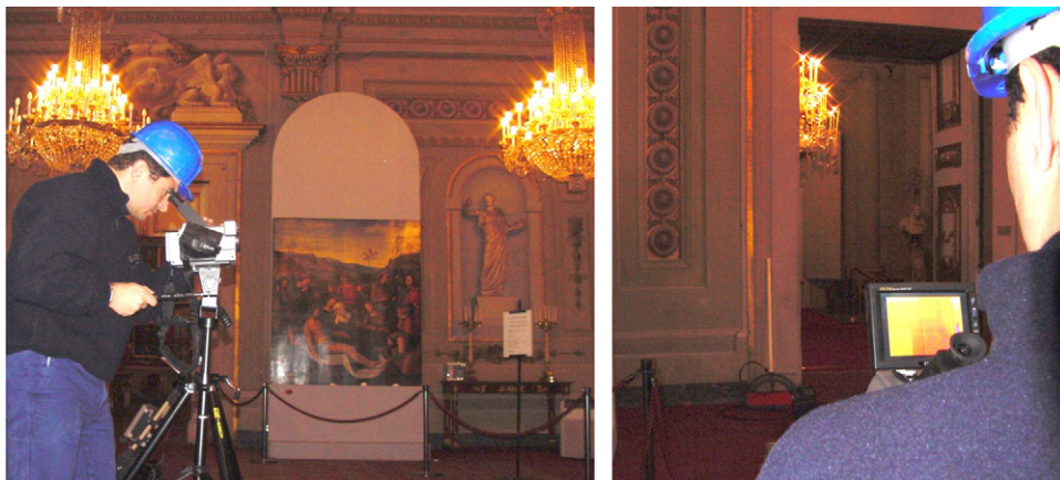
Fig. 4. Pictures of the infrared thermographic survey inside the "Sala delle Nicchie".
