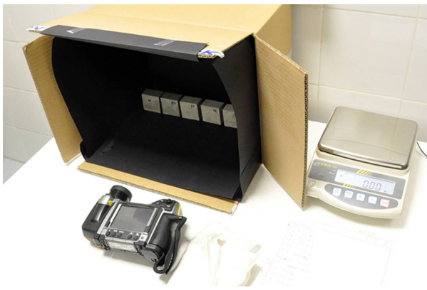
FIGURE 4. Equipment required for thermographic imaging and sample weight.
