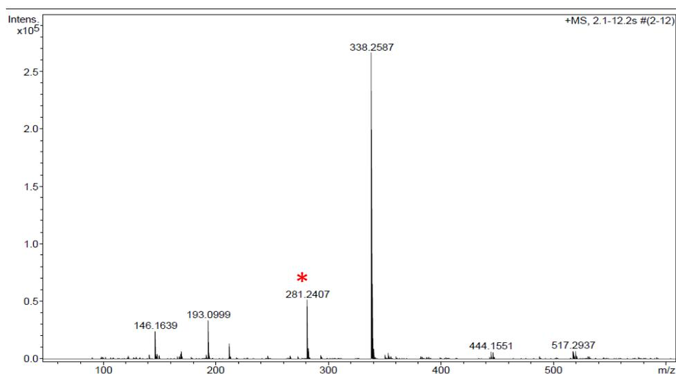
**Scheme 25.** HRMS (ESI-MS) spectrum of the product **P2**. Experiment performed in  $\text{CD}_3\text{CN}$ . \*The peak of  $m/z = 281.2407$  corresponds to **P5**.
