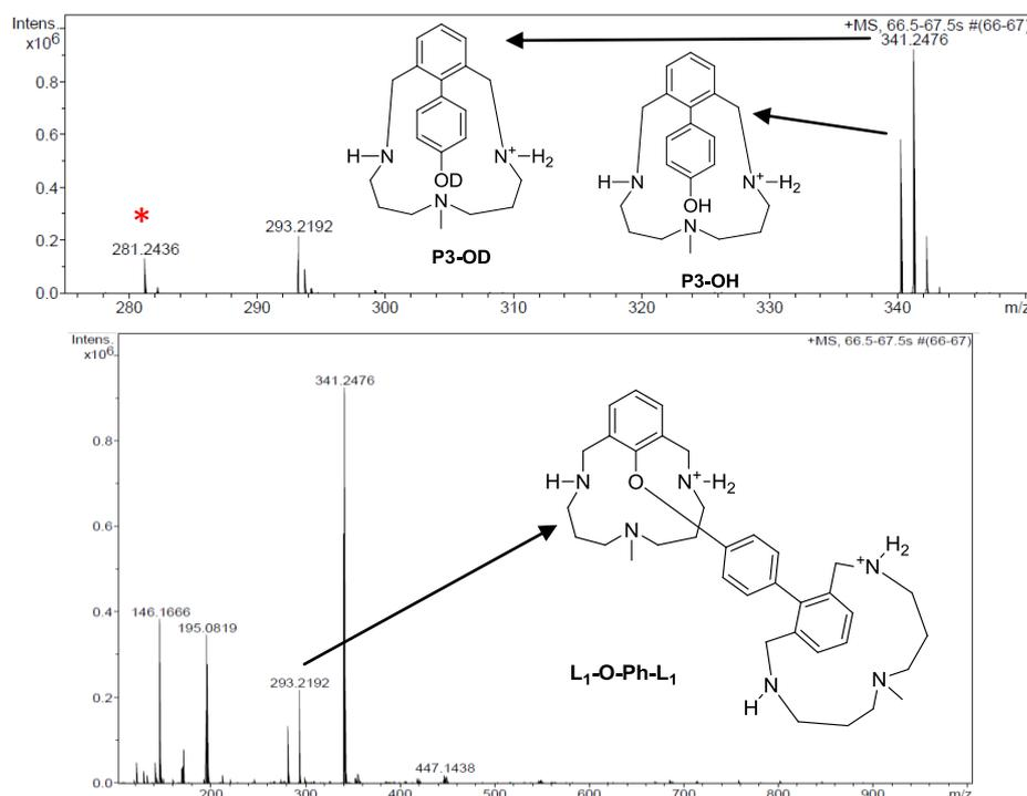
**Scheme 27.** HRMS (ESI-MS) spectrum of the product **P3-OH/OD** and **L1-O-Ph-L1**. Experiment performed in  $\text{CD}_3\text{CN}$ .
