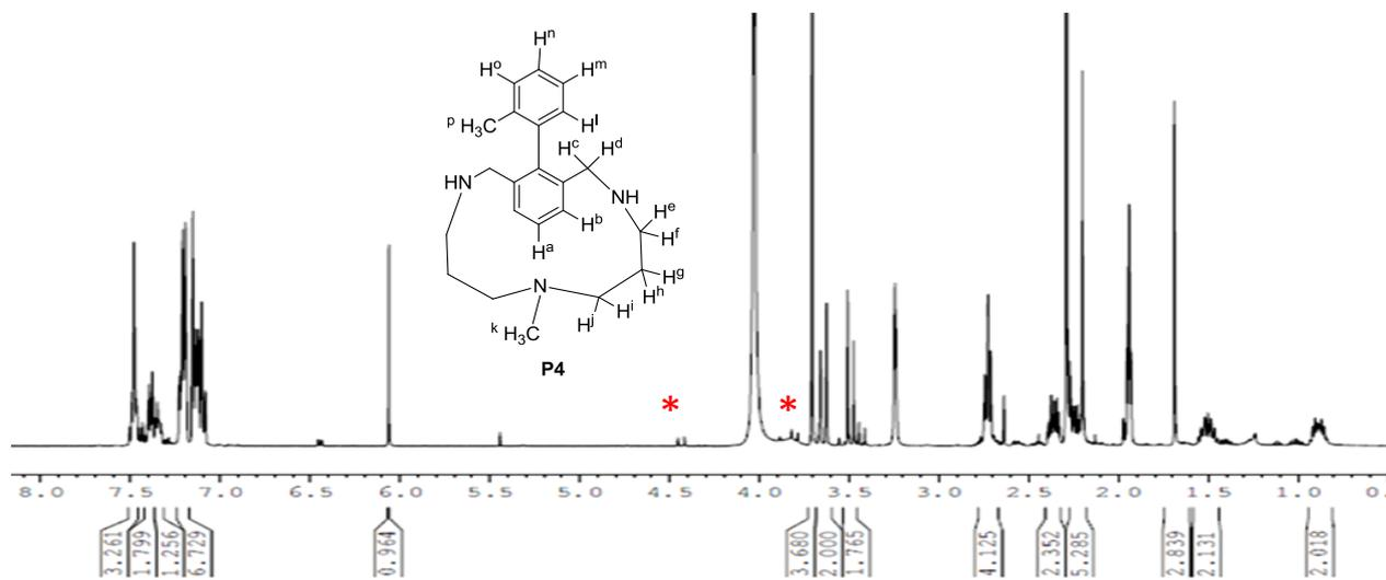
**Scheme 28.**  $^1\text{H}$ -NMR spectrum of compound **P4**. Experiment performed in  $\text{CD}_3\text{CN}:\text{CD}_3\text{OD}$ , 400 MHz, at 298 K. \*Impurities due to the product (**P5**) resulting from the insertion of methanol (solvent), that acts as a nucleophile (see section 4.3, where product **P5** is characterized).
