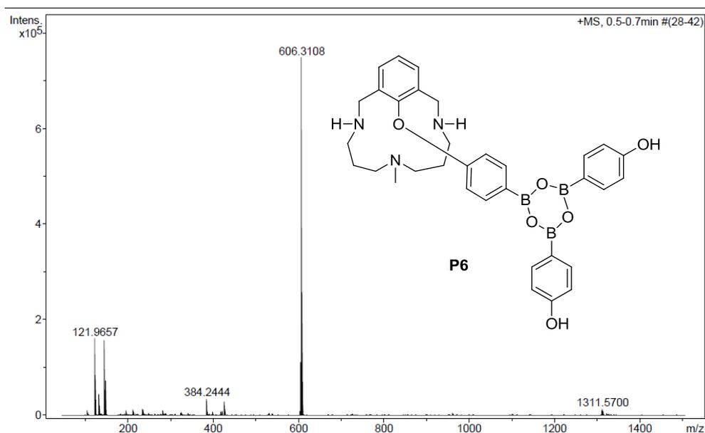
**Scheme 30.** HRMS (ESI-MS) spectrum of the product **P6**. Experiment performed in CD<sub>3</sub>CN.
