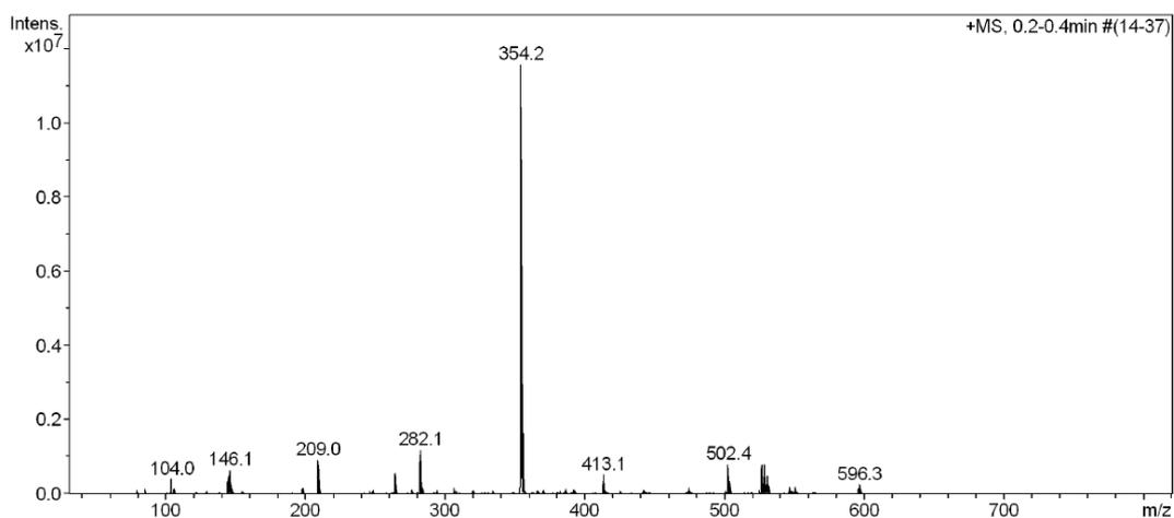
**Scheme 32.** ESI-MS spectrum of the product **P1**. Experiment performed in  $\text{CD}_3\text{CN}$ .
