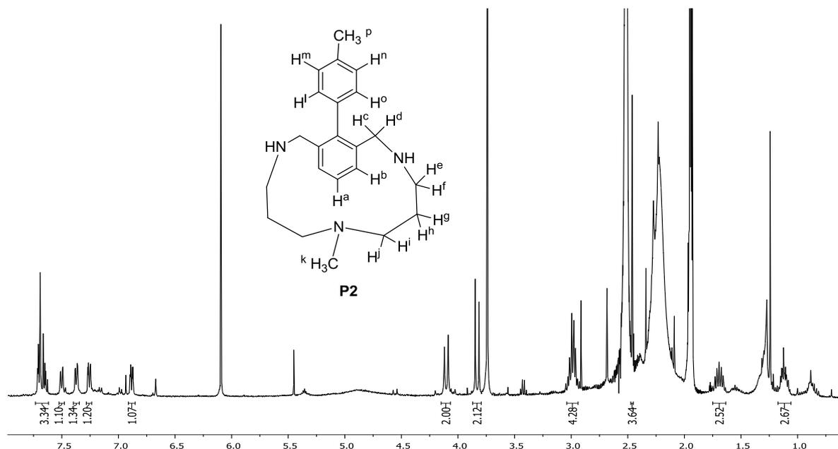
**Scheme 33.**  $^1\text{H-NMR}$  spectrum of compound **P2**. Experiment performed in  $\text{CD}_3\text{CN}$ , 400 MHz, at 298 K.
