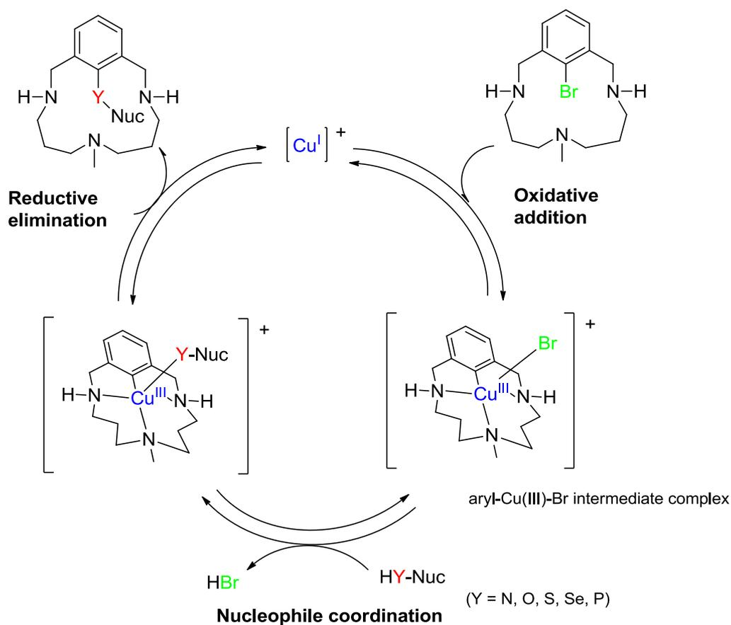
**Scheme 9.** Cu-catalyzed C-heteroatom cross-coupling reaction using a model aryl halide substrate.
