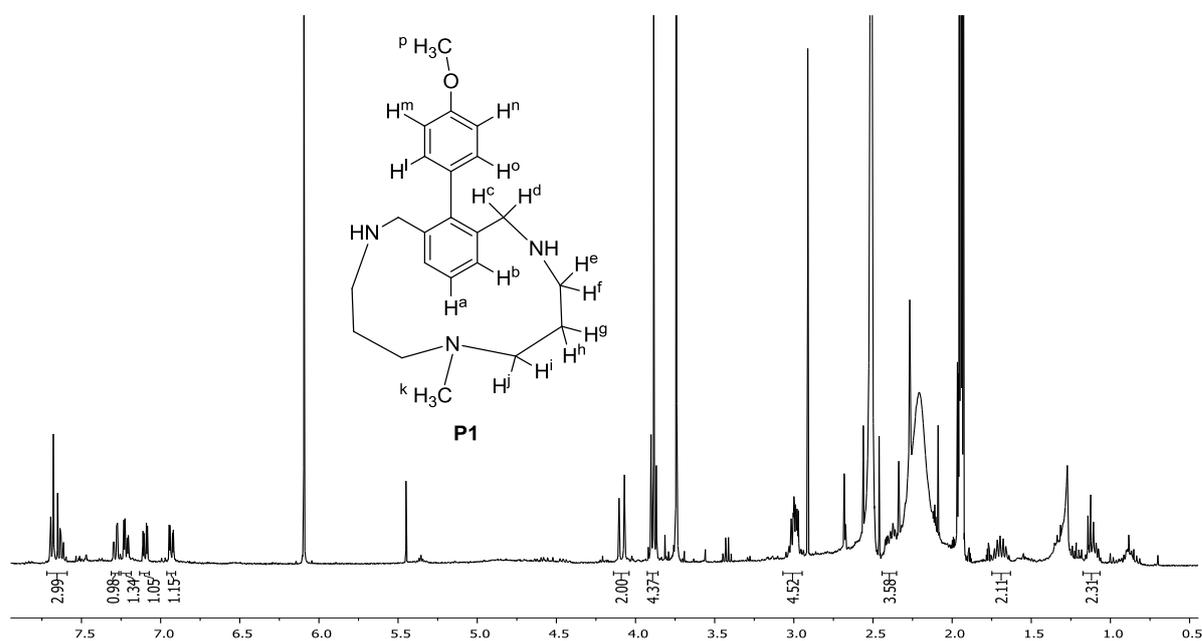
**Scheme 31.**  $^1\text{H-NMR}$  spectrum of compound **P1**. Experiment performed in  $\text{CD}_3\text{CN}$ , 400 MHz, at 298 K.
