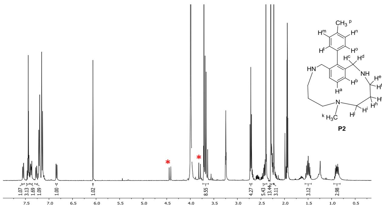
**Scheme 24.**  $^1\text{H-NMR}$  spectrum of compound **P2**. Experiment performed in  $\text{CD}_3\text{CN}:\text{CD}_3\text{OD}$ , 400 MHz, at 298 K. \*Impurities due to the product (**P5**) resulting from the insertion of methanol (solvent), that acts as a nucleophile (see section 4.3, where product **P5** is characterized).
