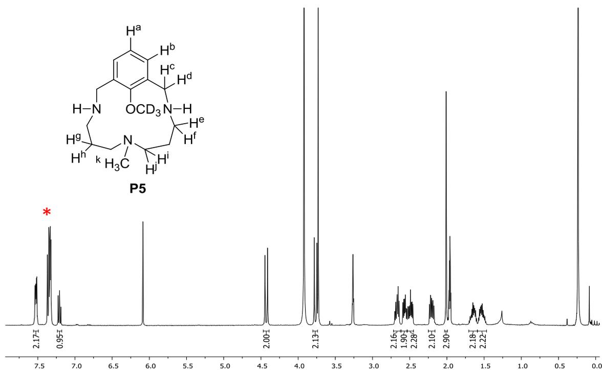
**Scheme 38.**  $^1\text{H-NMR}$  spectrum of compound **P5**. Experiment performed in  $\text{CD}_3\text{CN}:\text{CD}_3\text{OD}$ , 400 MHz, at 298 K using trimethyl(phenyl)silane as a transmetallating agent (Table 3, entry 1). \*Impurities due to the excess of the arylsilane.
