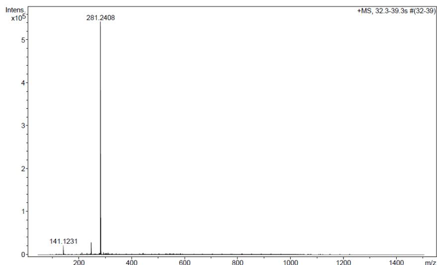
**Scheme 39.** HRMS (ESI-MS) spectrum of the product **P5**. Experiment performed in  $\text{CD}_3\text{CN}$ .
