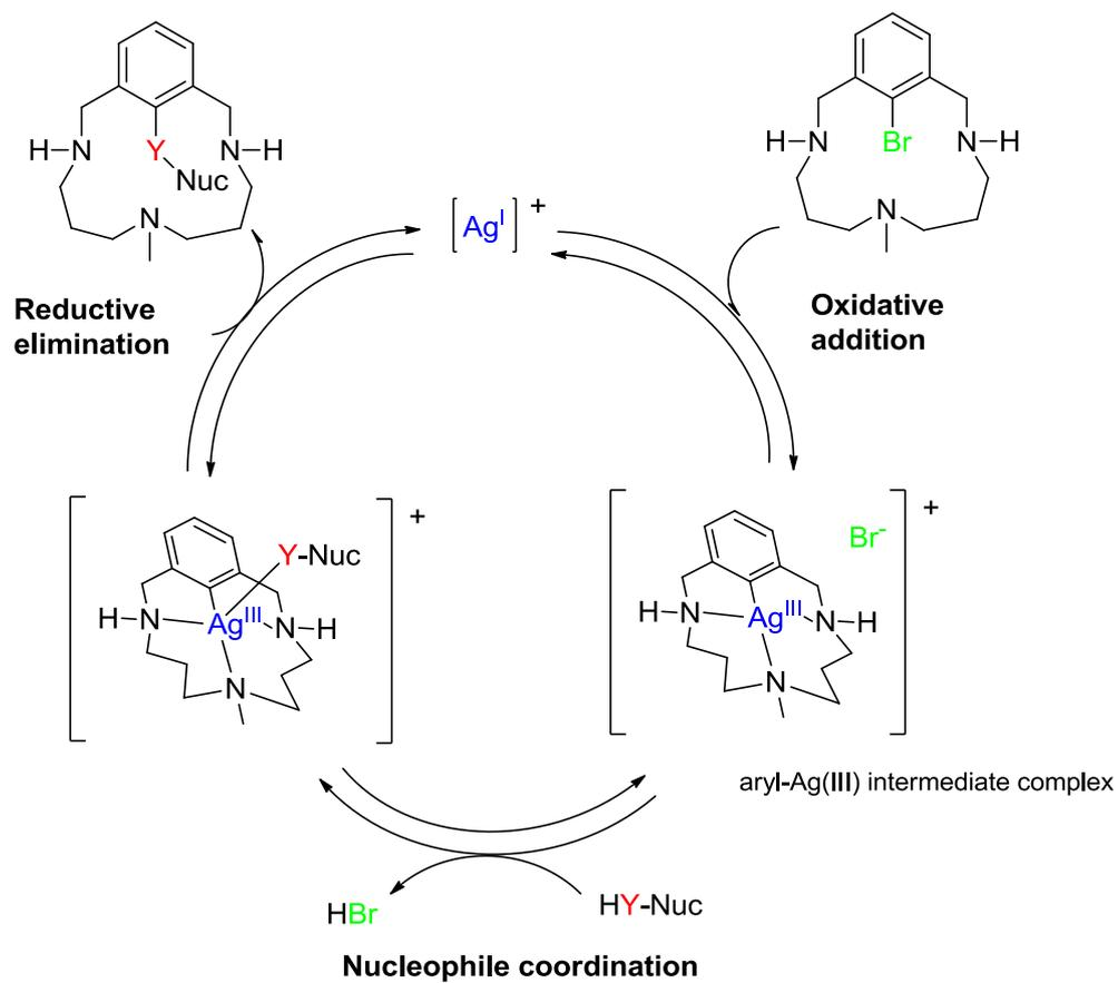
**Scheme 10.** General proposed mechanism of Ag(I)-catalysed cross-coupling reactions through the intermediacy of an aryl-Ag(III) complex using a model aryl halide substrate.
