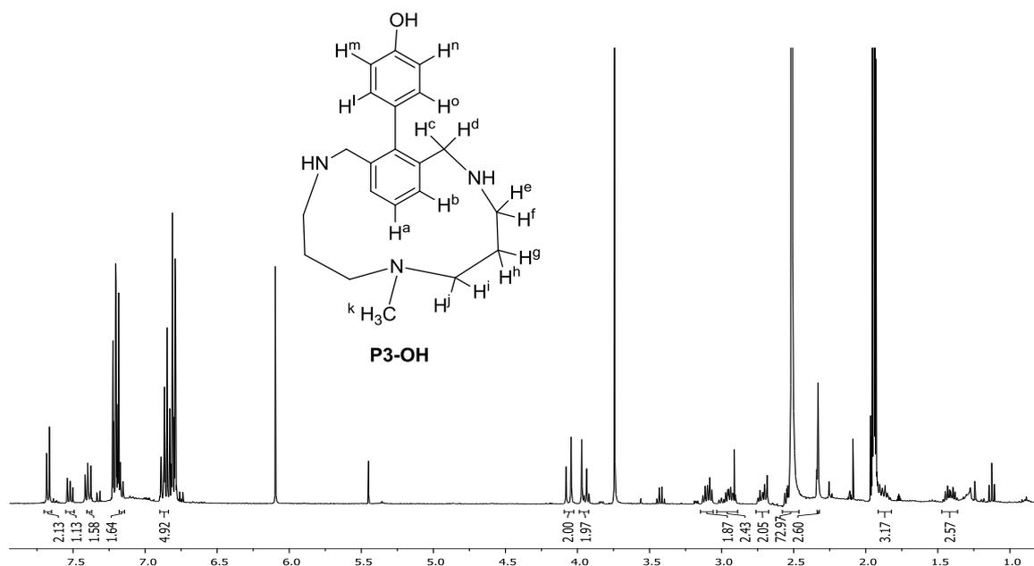
**Scheme 35.**  $^1\text{H-NMR}$  spectrum of compound **P3-OH**. Experiment performed in  $\text{CD}_3\text{CN}$ , 400 MHz, at 298 K.
