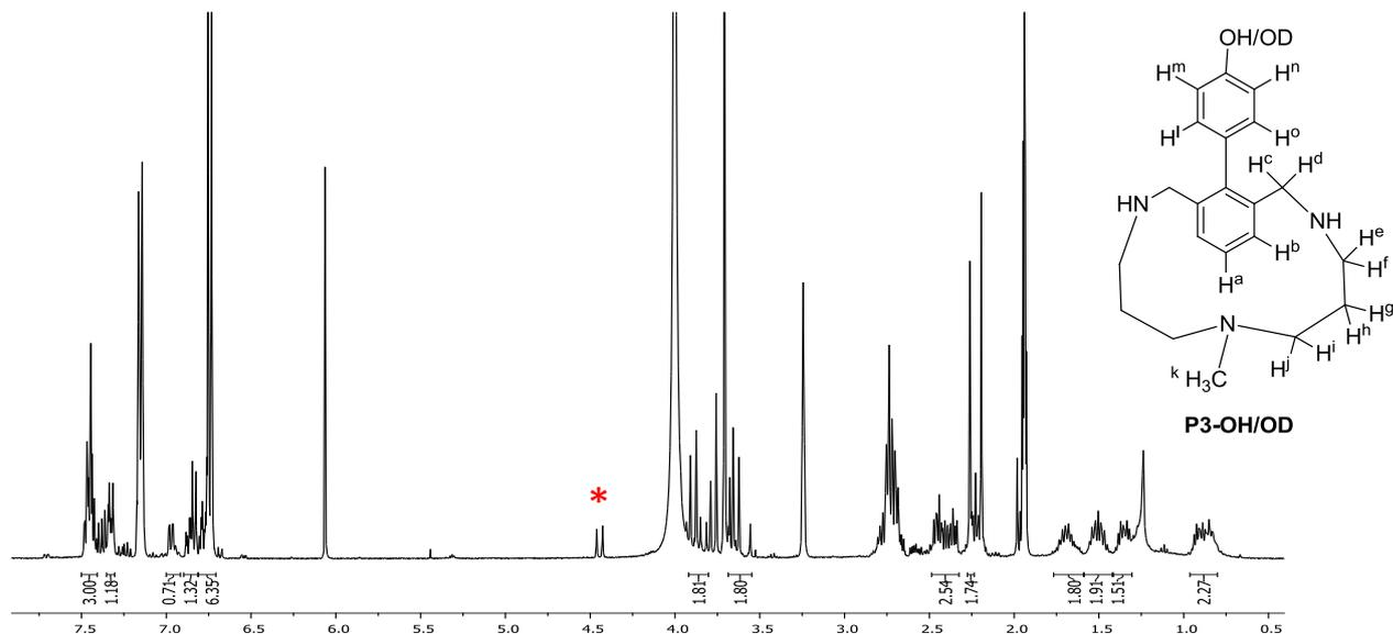
**Scheme 26.**  $^1\text{H-NMR}$  spectrum of compound **P3-OH/OD**. Experiment performed in  $\text{CD}_3\text{CN}:\text{CD}_3\text{OD}$ , 400 MHz, at 298K.
