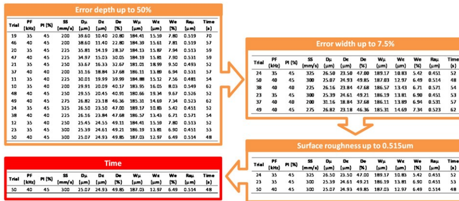
Fig. 7. Example of the multi-criteria selection process for the cDepth (up to 50%) - cWidth (up to 7.5%) - R_a (up to 0.515 \mu\text{m} ) - time.
