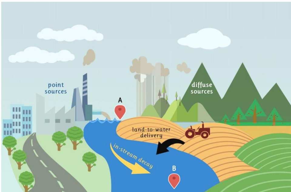
Figure 1: The SPARROW model relates measured nutrient flux (i.e., monitoring points A and B) in rivers and streams to watershed characteristics associated to nutrient sources (point and diffuse) and to nutrient mobilization and decay processes (land-to-water delivery and in-stream decay).
