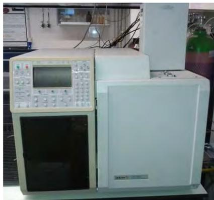
**Figure 3.7** Picture of gas chromatograph (CP-3800)
