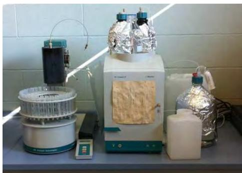
**Figure 3.11** Picture of ion chromatography (Metrohm 761-Compact)
