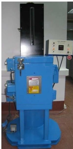
**Figure 3.12** Picture of gamma irradiator
