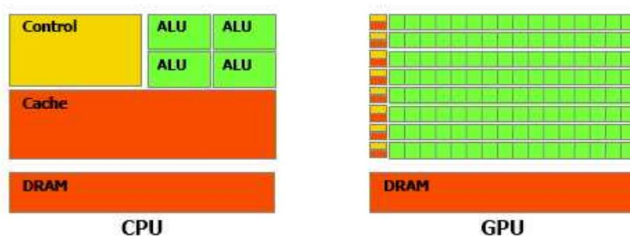
Figure 1.5: CPU and GPU Architecture. GPU devotes more transistors to data processing. Taken from [111].
