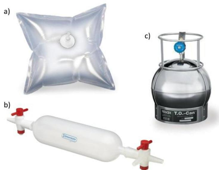
**Figure 1.3.** Examples of some types of containers used for sampling odour-causing compounds: a) Sampling bag, b) glass sampling bulb, c) canister.
