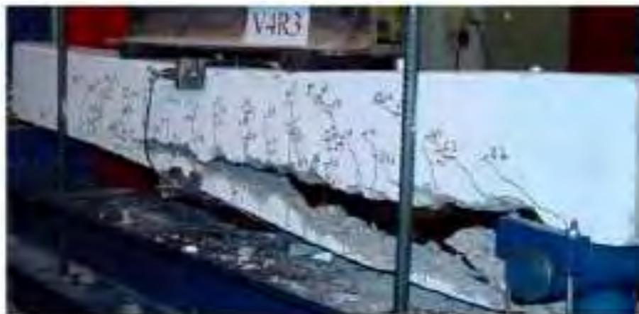
Figure 2.15: Failure mode of the tested beams [21].
