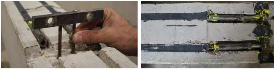
(a) End supporting mechanism for specimen MB2C1ES
