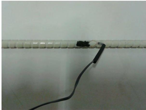
Figure 6.11: Strain gauges on the NSM bars.
