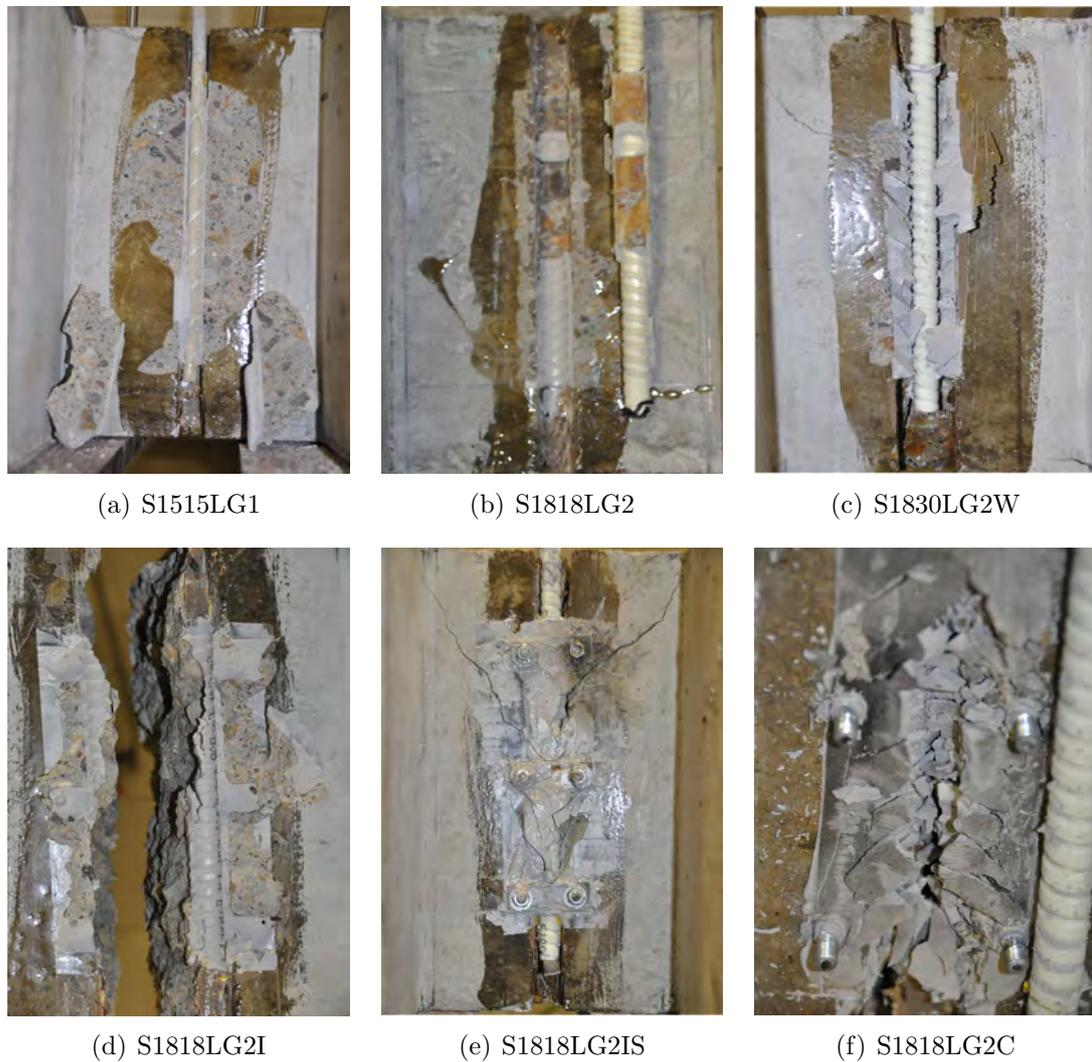
Figure 4.5: Modes of failure of specimens with GFRP bars.
