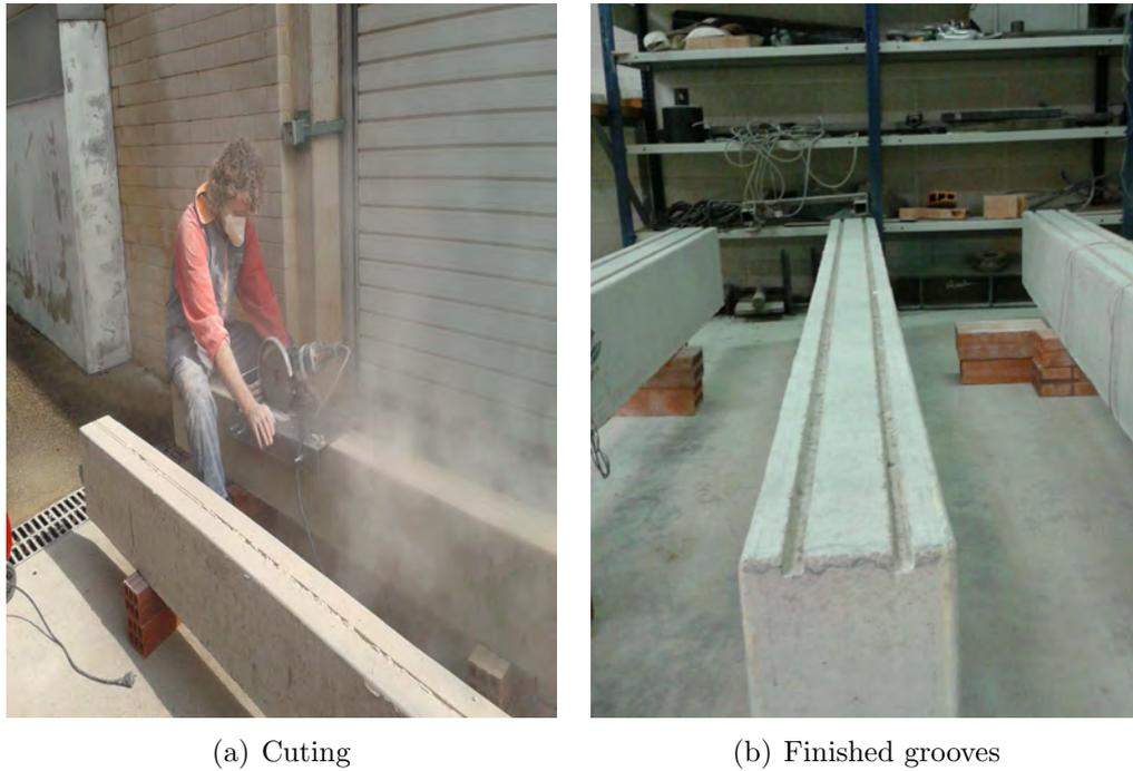
Figure 6.4: Formation of the grooves in the tension side of beams.
