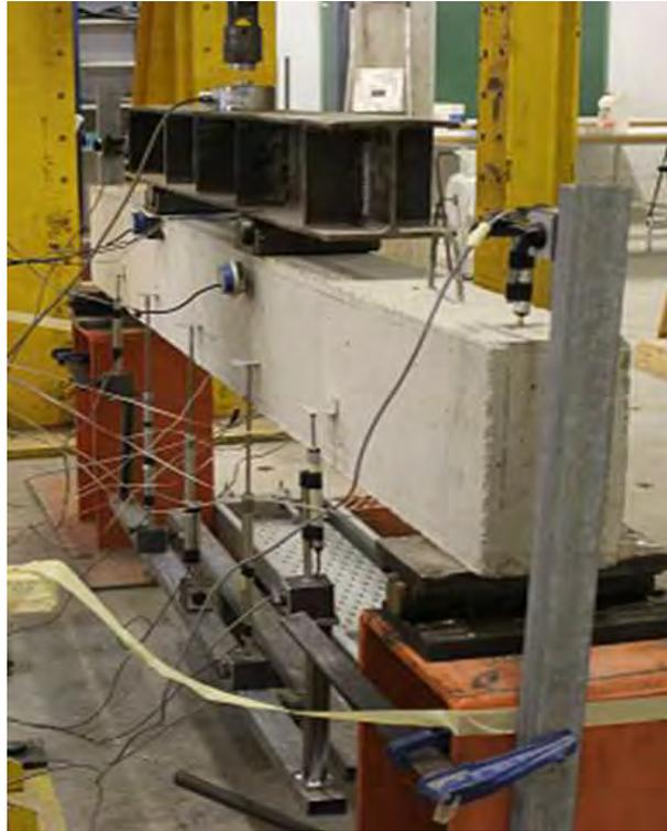
Figure 6.9: Arrangement of the vertical transducers and inclinometers.
