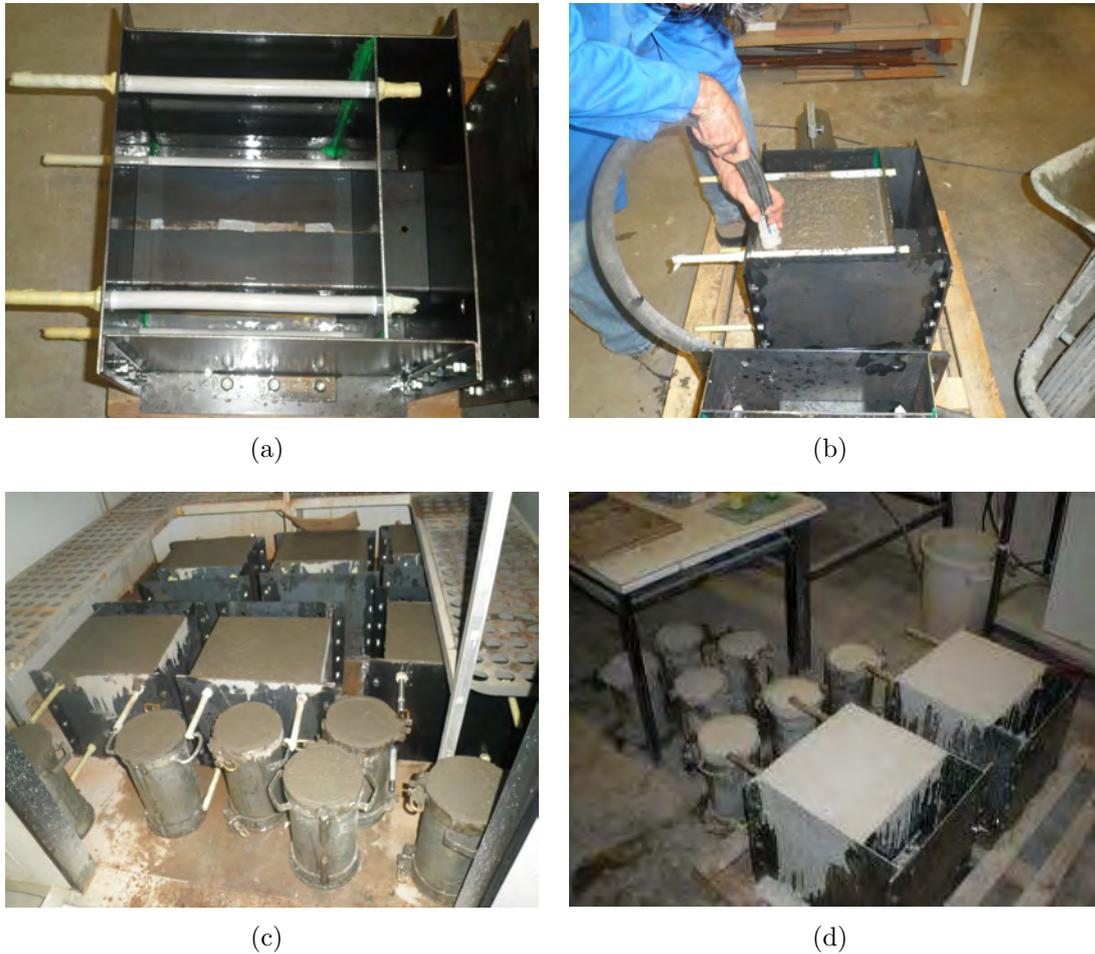
Figure 3.3: Mould preparation and casting.
