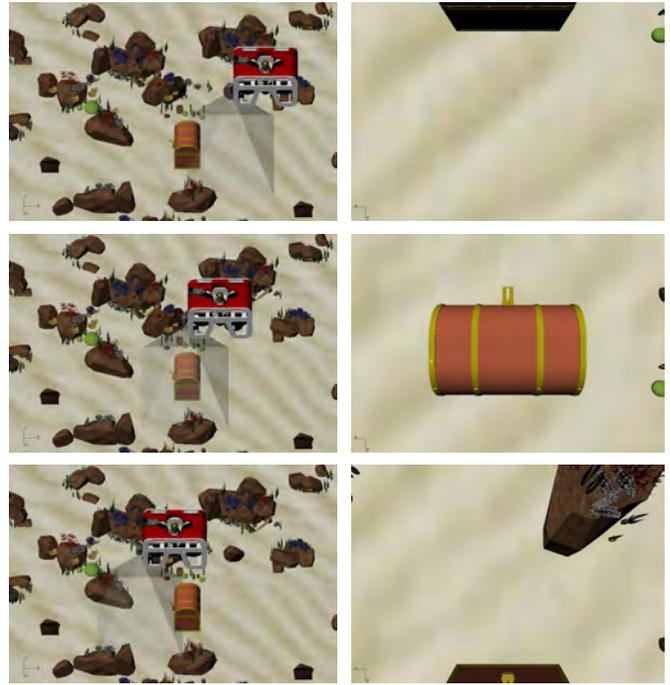
Fig. 1. Sequence corresponding to a straight trajectory of an AUV depicting the parallax problems. It shows the side and camera views of the robot's trajectory. One side of the chest disappears from the frame while the other arises due to the parallax effect.
