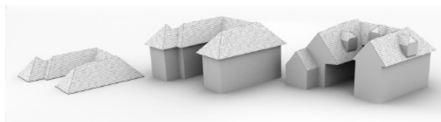
Fig. 32. Left: Straight skeleton; Middle: Straight Skeleton with angle changes; Right: Procedural extrusions
