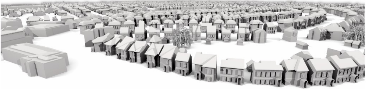
Fig. 2. We present an interactive procedural modeling system that is able to model difficult architectural surfaces, such as roof constructions. This figure shows procedural extrusions applied to 6000 floorplans from a GIS database of Atlanta.
