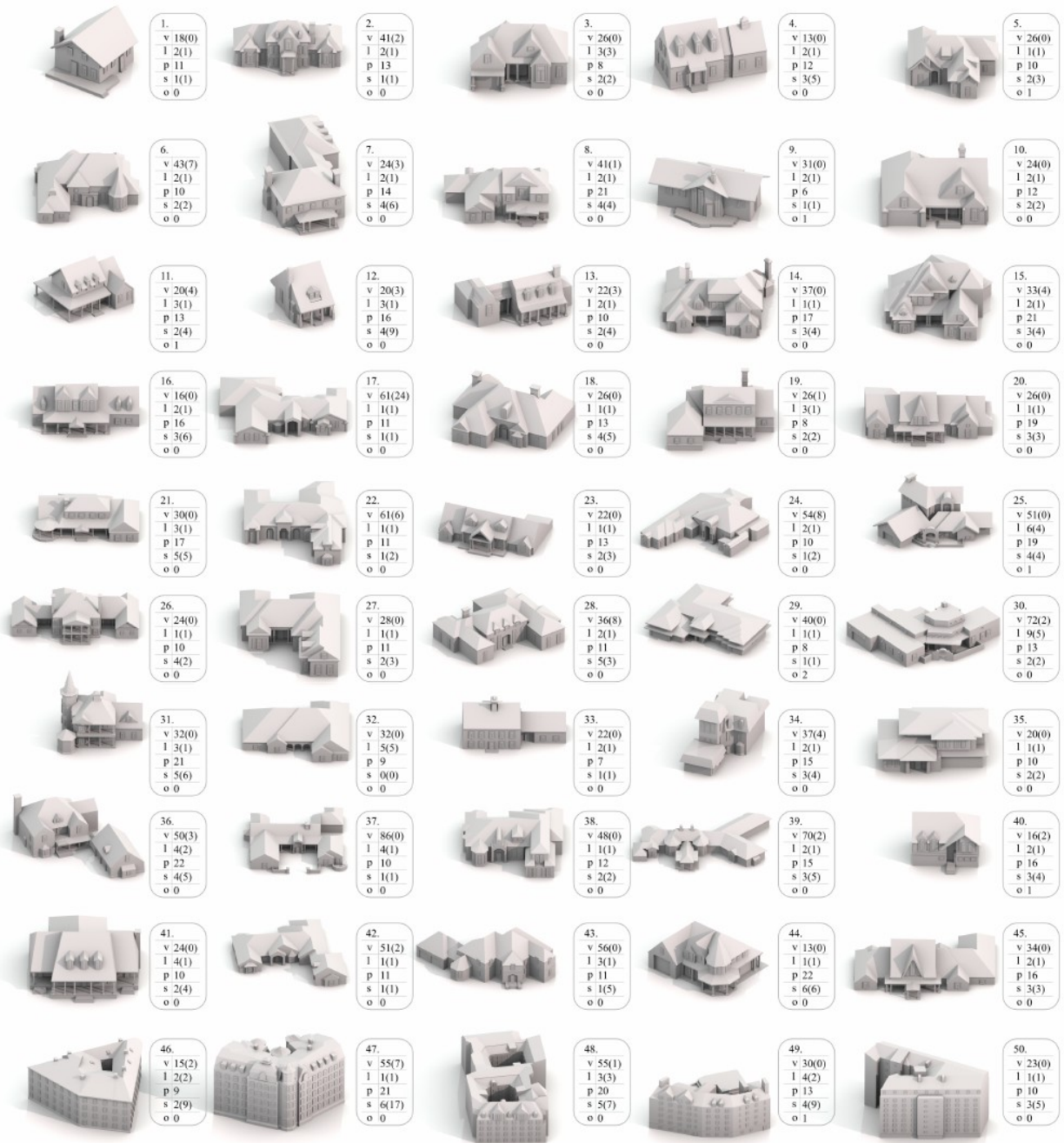
Fig. 25. The example cases and modeling statistics. v Vertices in modeled plan (additional vertices); l Polygons in modeled plan (polygons in library plan); p Number of profile sections in model; s Number of natural steps designed (number of natural step applications); o Number of offset events.
