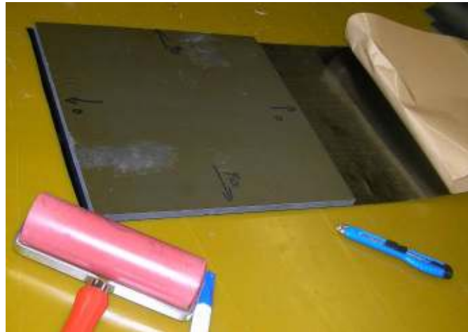
Fig. 3.11. Cutting pattern and roller used for proper stacking
