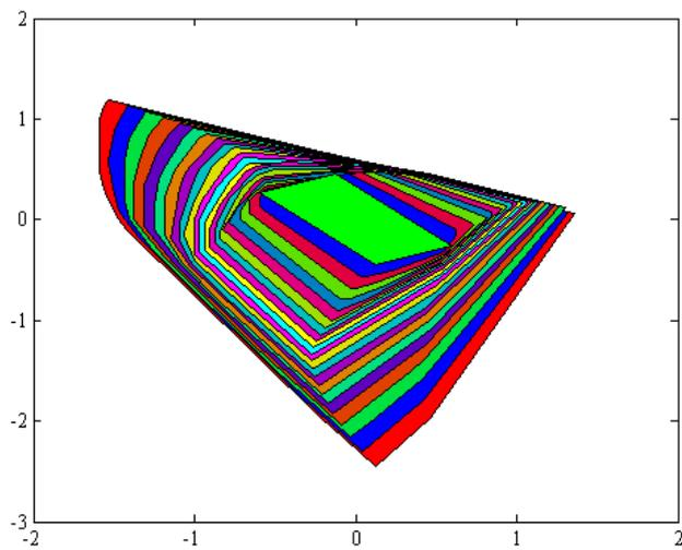
Figure 6.4: The computed polytopic robust controllable sets with  $\varepsilon = 0.05$
