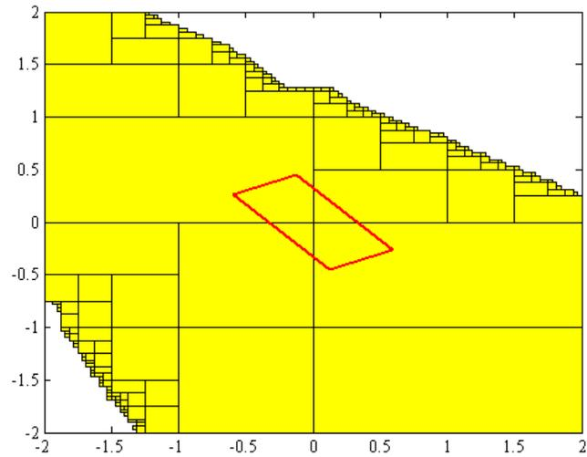
Figure 5.5: The inner approximation of the maximal robust controllable set
