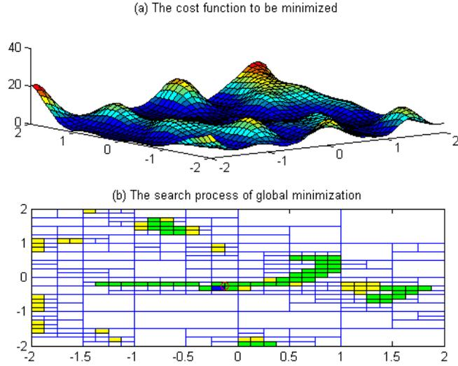
Figure 4.2: An example of global minimization via interval analysis
