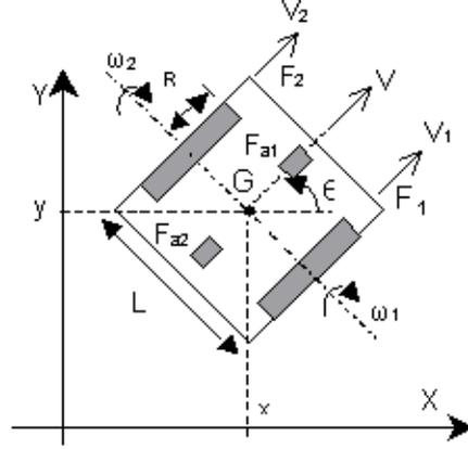
Figure 7.1: The configuration of the MiroSot robot
