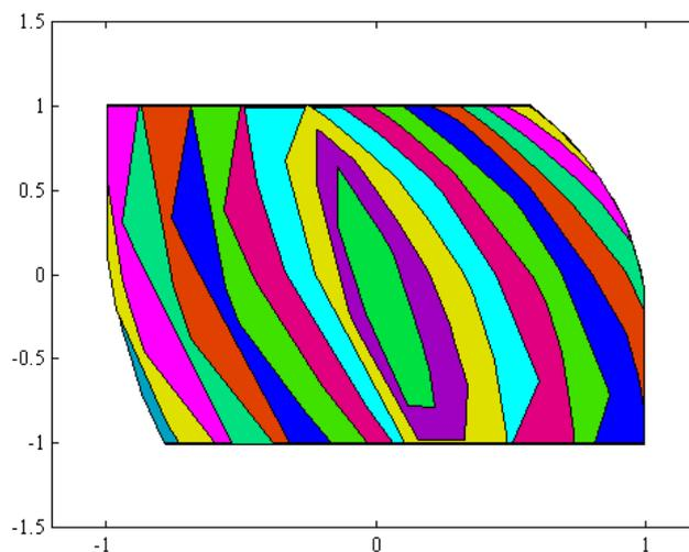
Figure 6.14: The polytopic quasi 2-step robust controllable set sequence
