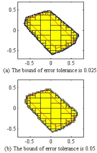
Figure 6.3: The first-step robust controllable sets with  $\varepsilon = 0.025$  and  $\varepsilon = 0.05$
