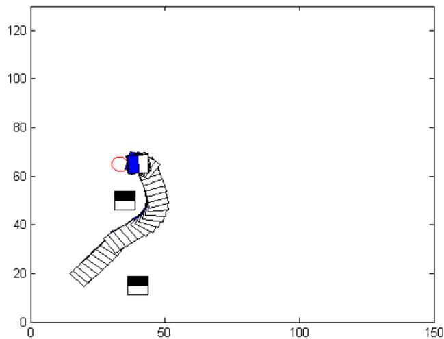
Figure 7.2: The control of a MiroSot robot with automatic obstacle avoidance
