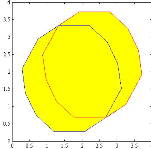
Figure 4.4: Bisection of a zonotope with redundant line segment generators
