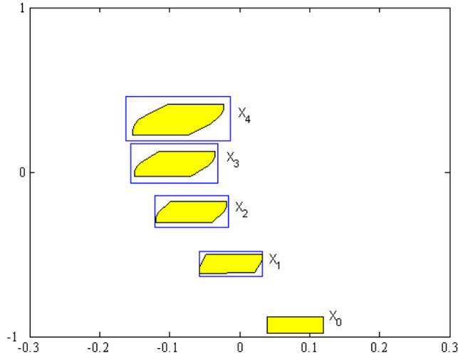
Figure 4.6: The zonotope evolution vs the interval evolution
