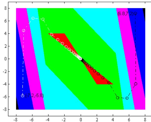
Figure 3.4: Linear contractive MPC with a contractive sequence of controllable sets
