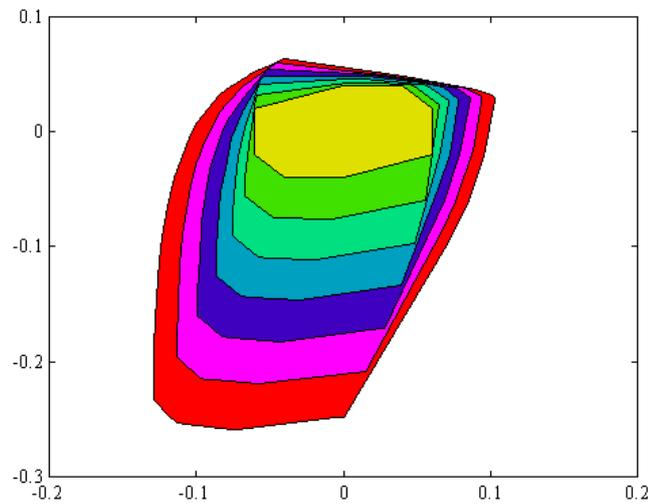
Figure 7.5: The computed polytopic controllable sets of the CSTR
