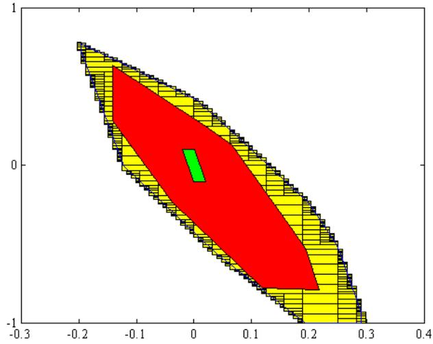
Figure 6.12: The terminal set, the quasi one-step set and its polytopic approximation
