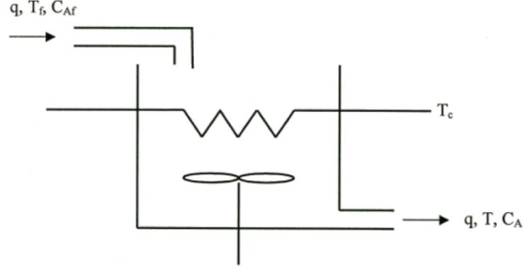
Figure 7.3: The configuration of the CSTR
