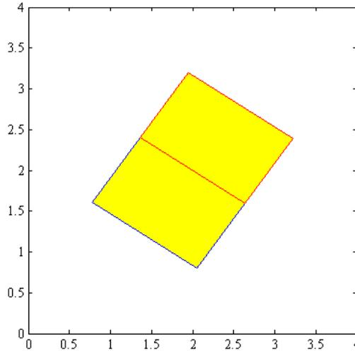
Figure 4.5: Bisection of a zonotope with linearly independent line segment generators
