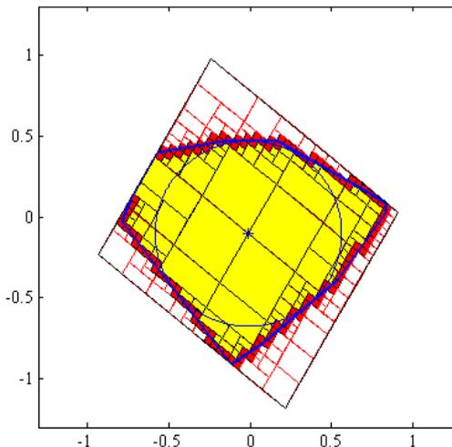
Figure 4.8: Inner approximation of a polytope by a union of zonotopes
