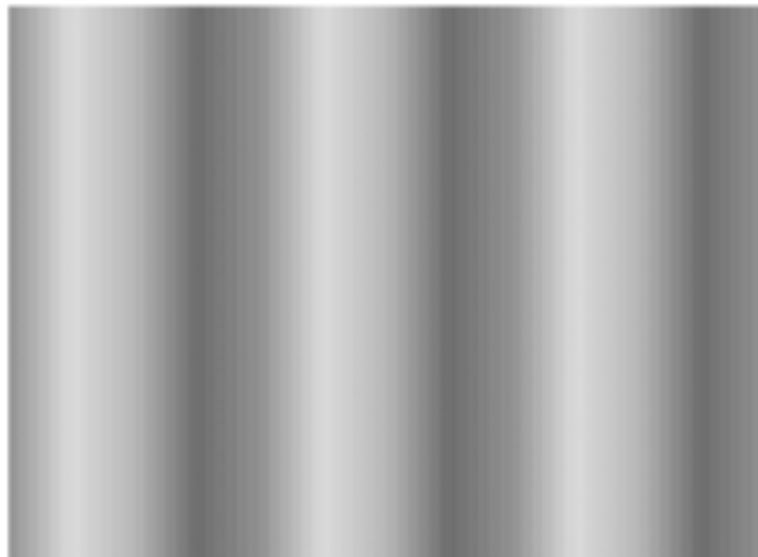
Figure 4.26: The periodical pattern proposed by Wust and Capson, made by the sinusoidal overlapping of the three primary colour components.
