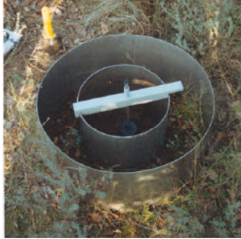
Figure 4.5. Example of a double-ring infiltrometer used for field determinations
