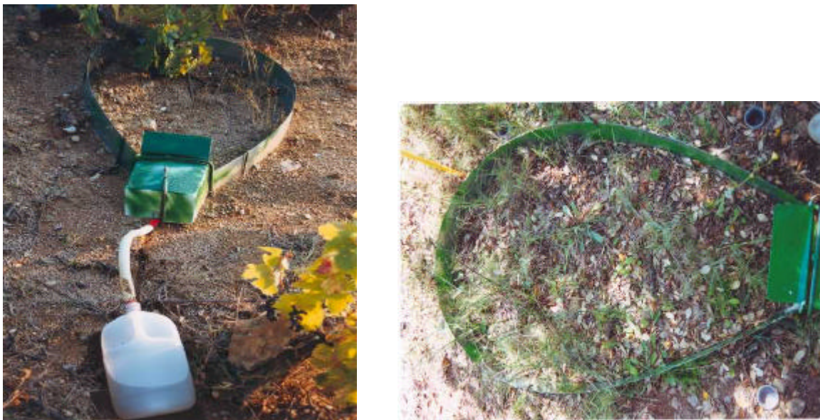
Figure 4.4. Example of a runoff-erosion microplot set up in a vineyard (left) and shrub environment (right).
