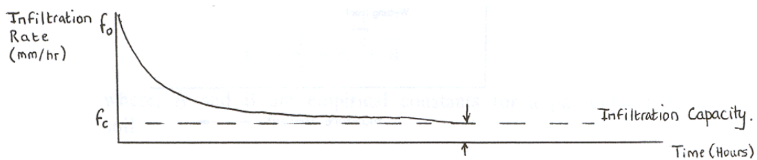
Figure 6.3. Horton's definition diagram for infiltration capacity
