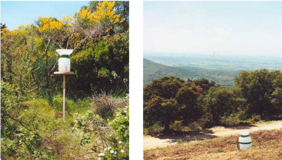
Figure 4.6. Example of a rain gauge of five-litre volume set up in a shrub environment (left); and one of 25 litre placed at the uppermost part of the study catchment (right).
