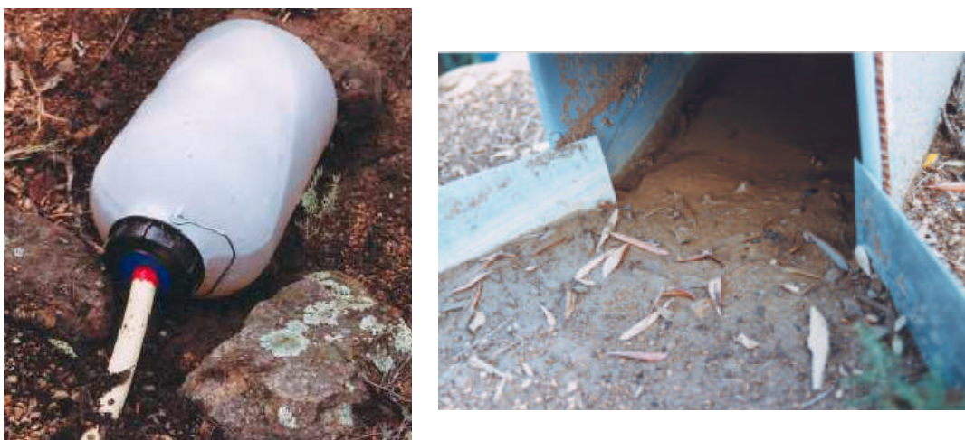
Figure 4.3. Runoff deposit (left) and sediment yield container (right) of a runoff-erosion microplot after a rainfall event.
