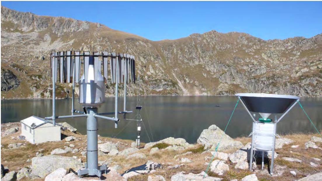
Figure 4. Atmospheric bulk deposition sampler, automatic weather station and field laboratory at Lake Redon, Central Pyrenees (by M. Bacardit).
