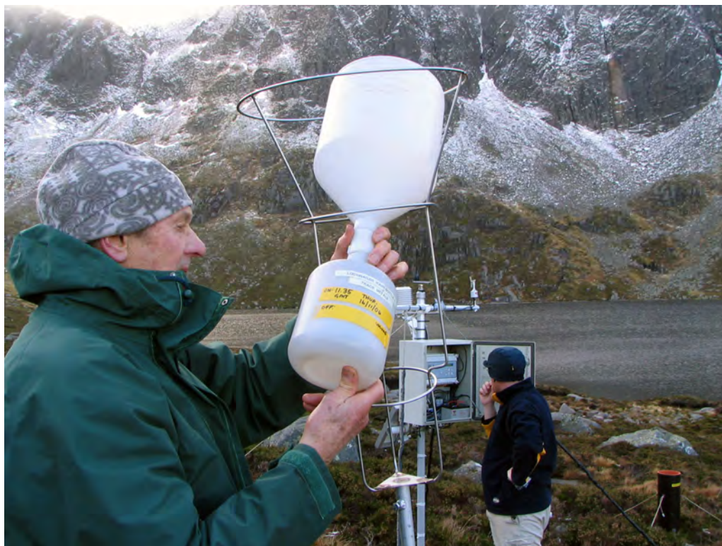
Figure 6. Atmospheric trace element deposition sampling at Lake Lochnagar, Grampian Mountains, Scotland (by M. Bacardit).
