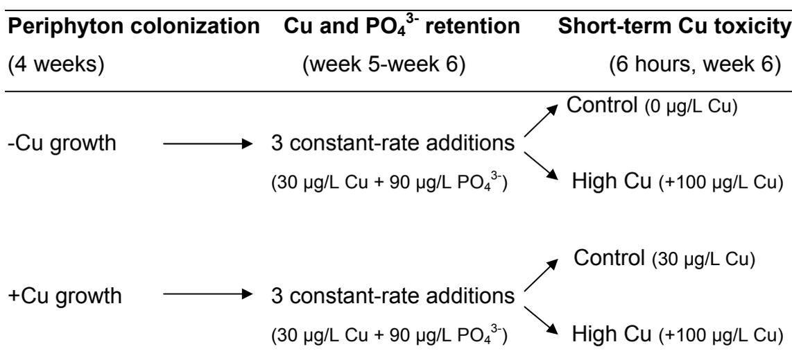
**Figure 2.** Scheme of the experimental setup including the duration and conditions (nominal concentrations) of each experiment
