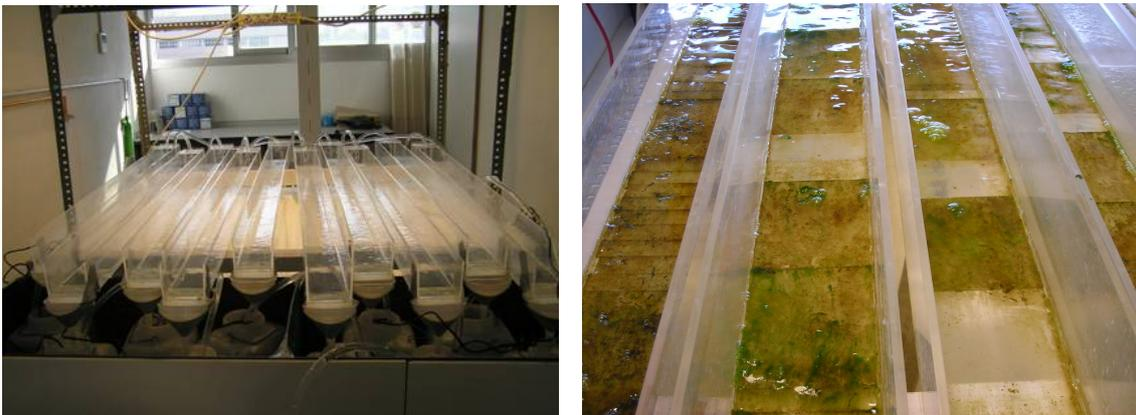
**Figure 2.** Picture of the experimental channel system without colonized substrata (left panel) and a detail of periphyton colonized substrata (right panel).
