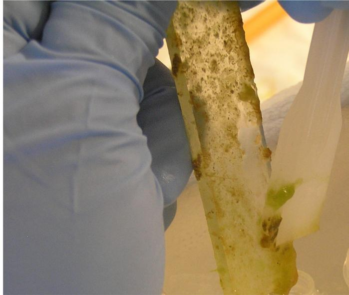
**Figure 3.** Detail of the periphyton scratching for Cu analysis.
